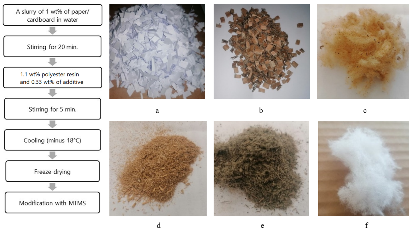
Figure 1 Aerogels production scheme; examples of aerogels raw materials and additives: (A) office paper; (B) cardboard; (C) wool; (D) straw; (E) algae; (F) cellulose acetate.
