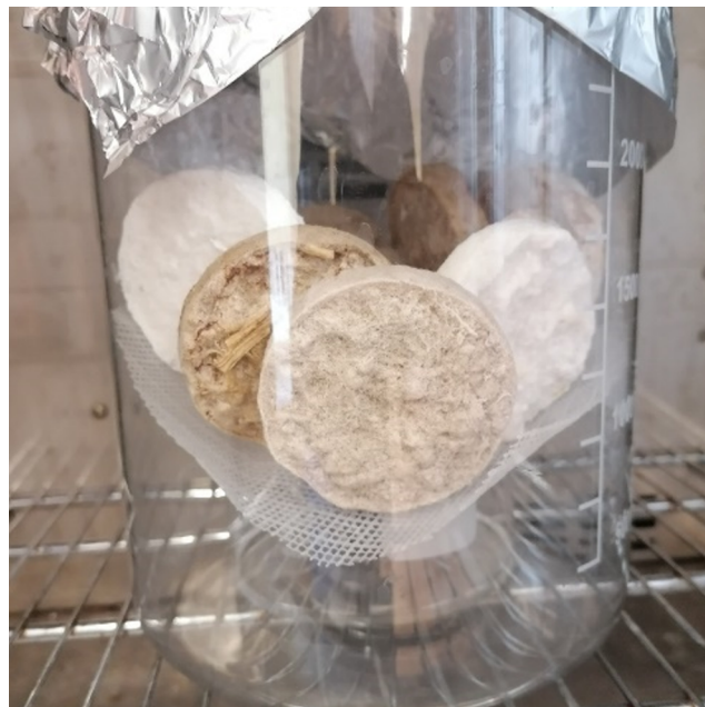
Figure 2 Photograph of an aerogel modification: aerogel samples of office paper are white, aerogel samples of cardboard are brownish. Full-size DOI: 10.7717/peerj.11795/fig-2
