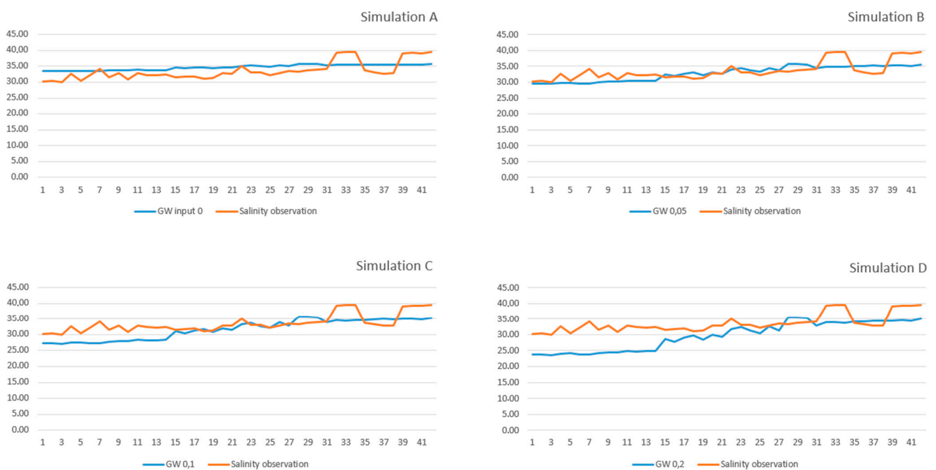
Figure 5. Modeled and observed salinity (PSU) comparison for each SGD input case (Simulation A): 0; (Simulation B): 0.05; (Simulation C): 0.1; (Simulation D): 0.2. With the x -axis representing the stations' numbers and the y -axis representing the salinity values.
