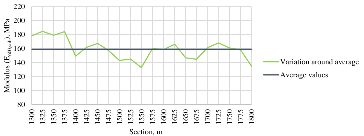
Fig 42. Subgrade's bearing capacity ( E_{600,sub} ) variation during the dry period on road No. 3118
