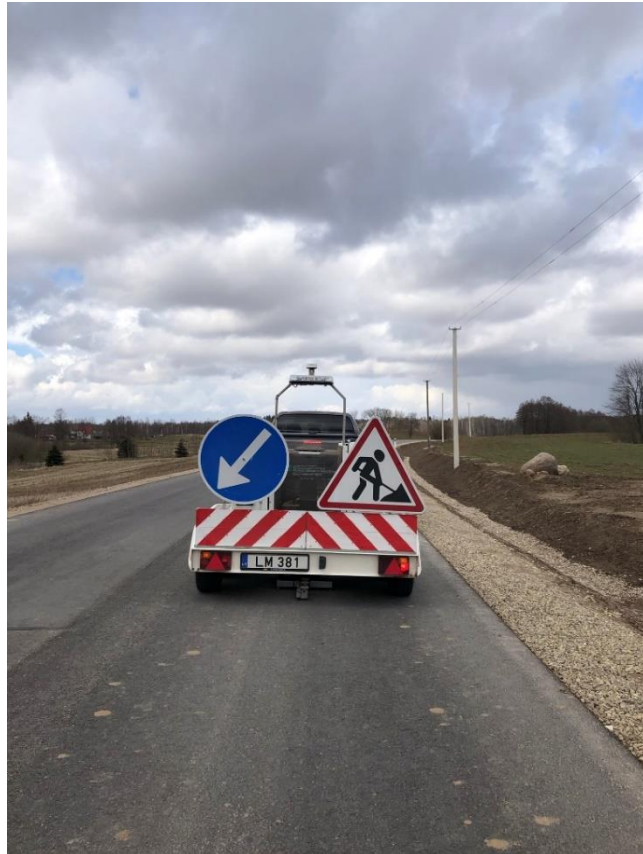
Fig 35. FWD test in the Regional road No. 1125
