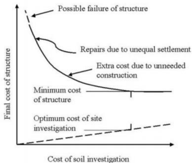
Fig 1. Effect of soil investigation on the final cost of structures
