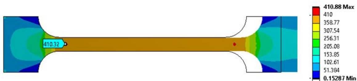
Figure 5 Test sample X: Max. Deformation 5.7807 mm; Von Mises equivalent stress 410.88 MPa
