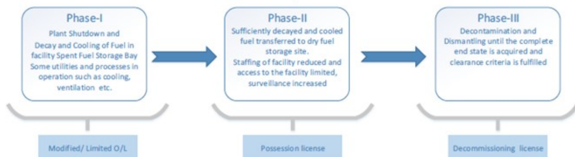
FIG.1 License conditions for different phases of decommissioning
