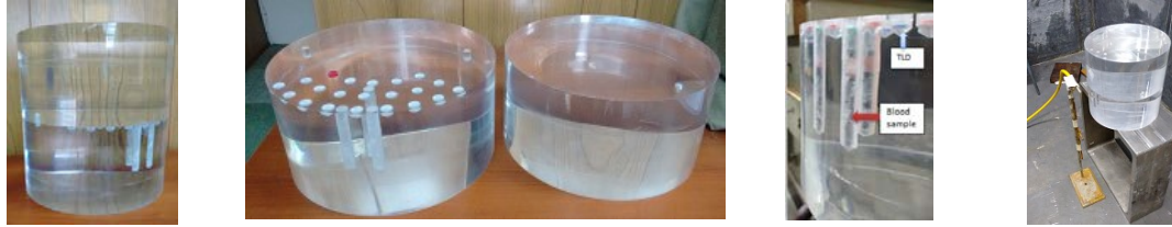
FIG. 4. Torso phantom with holes where TLDs and blood samples can be located for computational validation
