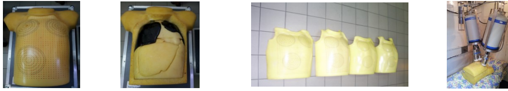
FIG. 3. LLNL realistic torso phantom, different chest plates and measurement geometry
