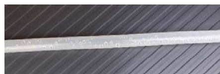
Fig. 5. Water vapour condensation inside the tubing which transported the gas sample between the beehive and the measurement device.
