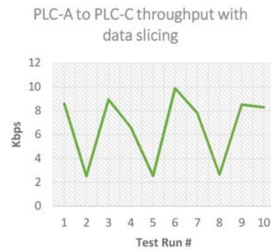
Fig. 6. Thresholds observed on PLC-A to PLC-C communication channel with data slicing at application level.
