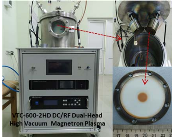
Fig. 1. The photos of the VTC-600-2HD DC/RF Dual-Head High Vacuum Magnetron Plasma System and the ZnO<La> sputtering target.
