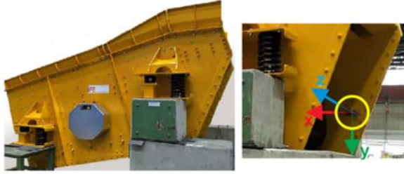
Fig. 4. Left: orbital vibration screen sieve placed in an experiment area which was monitored with the sensor module in Fig. 1. Right: Position of the sensor module on the inner side of the sieve (yellow circle) and orientation of sensor axis according to Fig. 3. In this test one axis of the sensor module was aligned close to the local horizon. Photo courtesy of IFE Aufbereitungstechnik GmbH, Waidhofen an der Ibbs, Austria.
