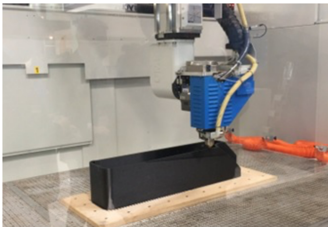
Figure 2 – 3D printing of carbon-composite compound (court. of CMS)
