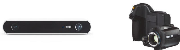
Figure 2 Sensors under investigation: Stereo camera ZED by STEREO LABS (left image) and Thermal camera T420 by FLIR (right image)
