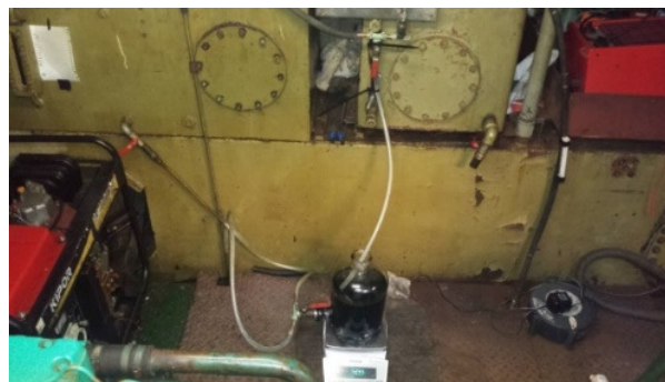
Fig. 3. The fuel measurement system, for fuel weight lost determination.
