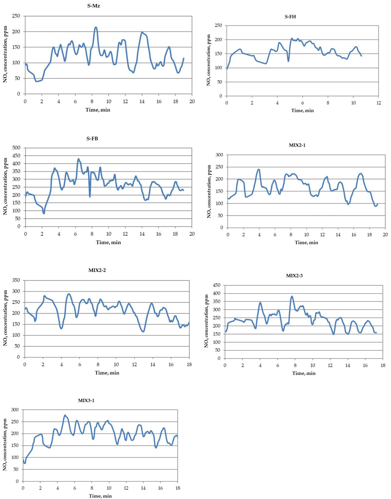
Figure 6. NO<sub>x</sub> concentrations during combustion of pellets.
