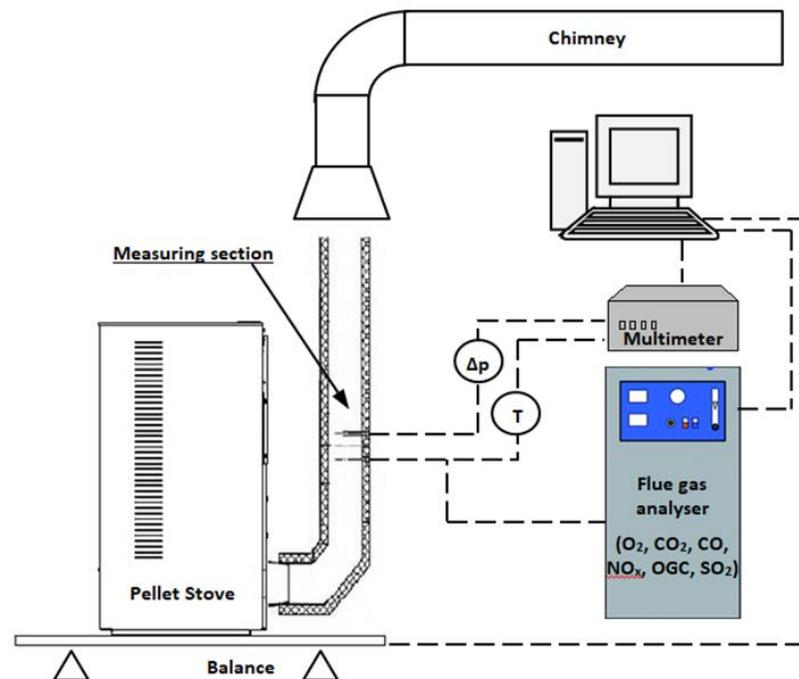
**Figure 1.** The schematic view of pellet combustion process.
