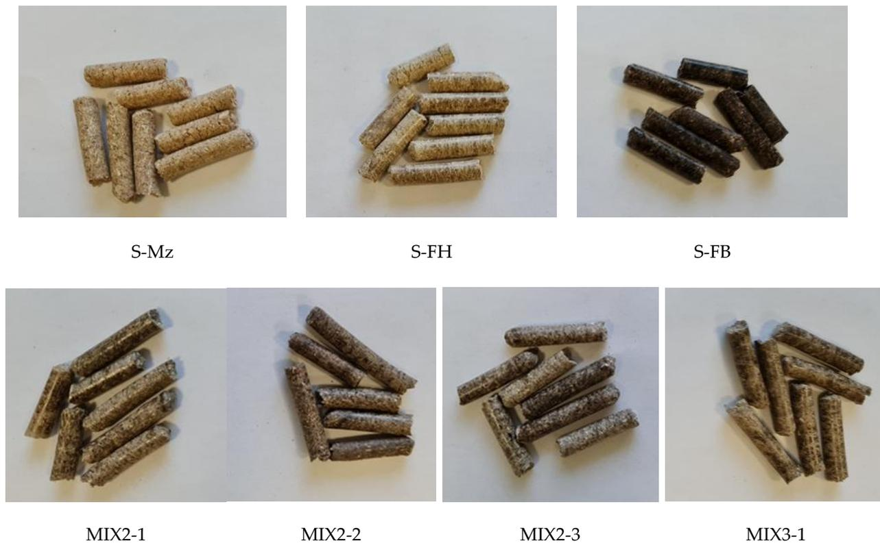
**Figure 2.** Samples of produced pellets.
