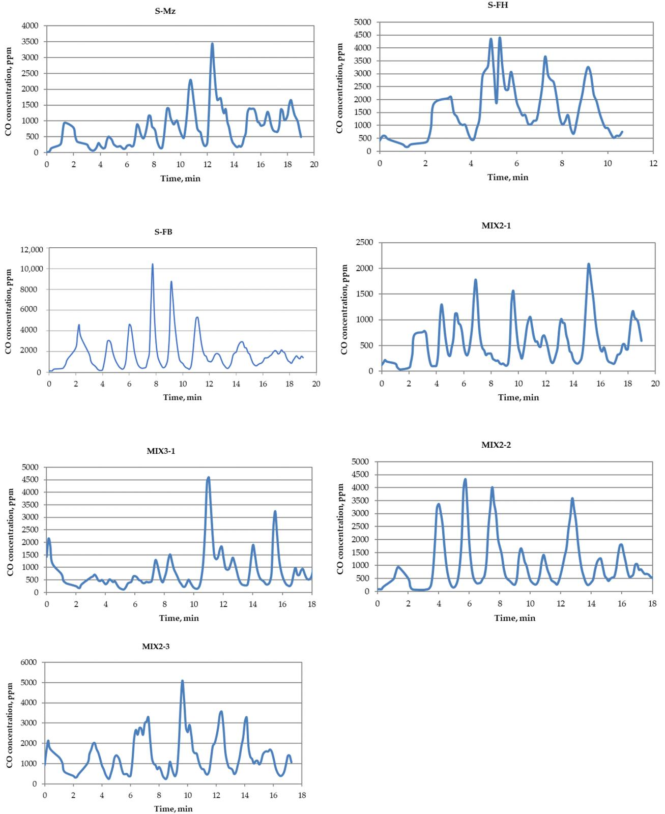
Figure 5. CO concentrations during combustion of plant biomass pellets.
