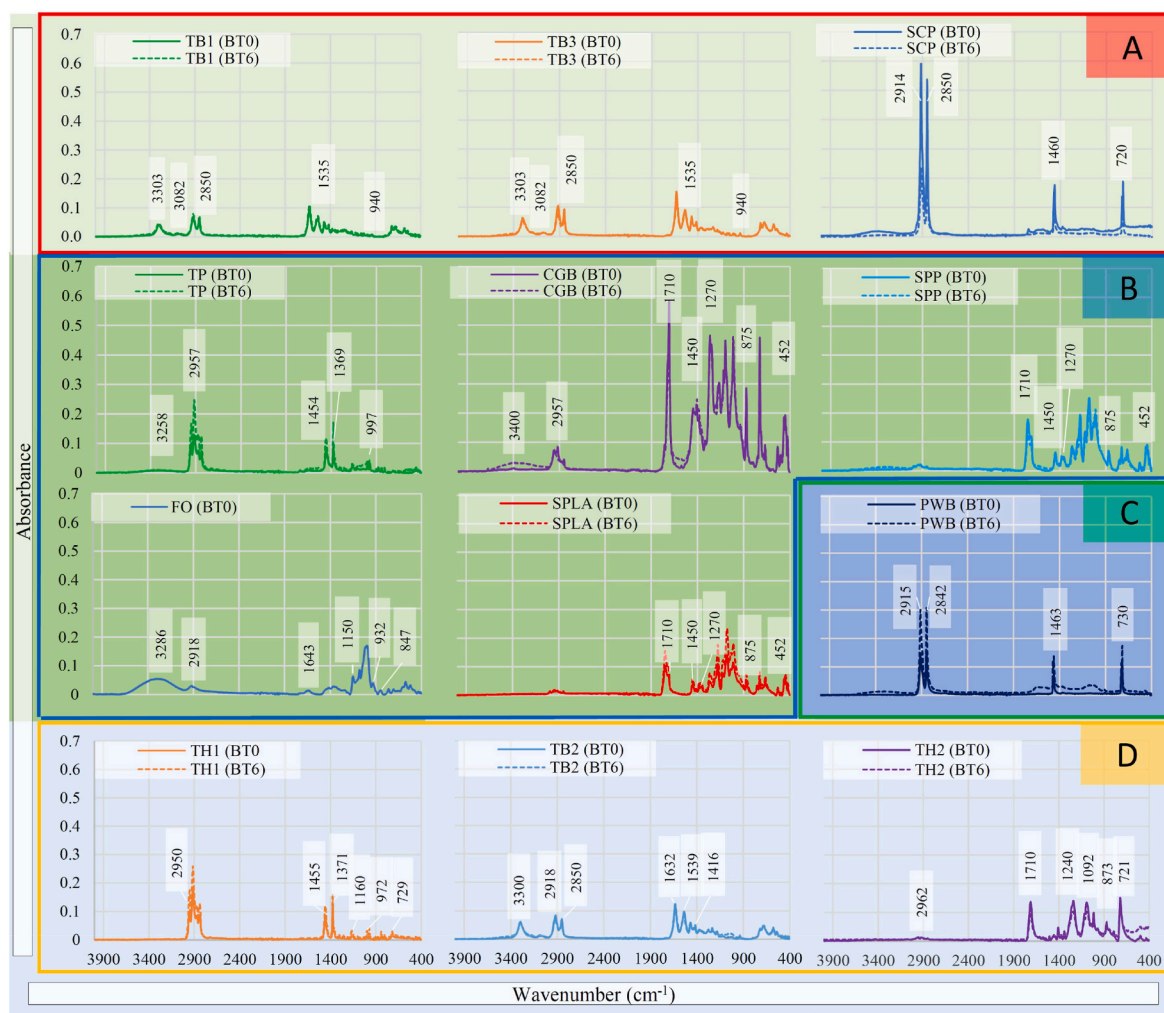
Fig. 7. ATR-FTIR spectra of raw (BT0) and treated (BT6) samples.
