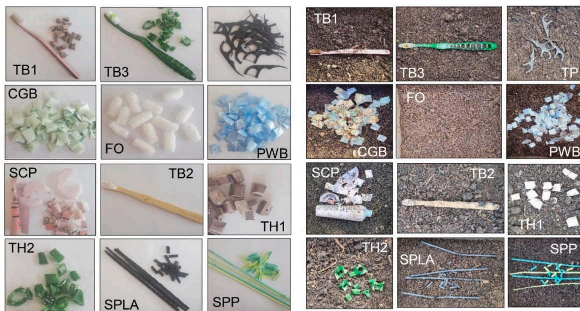
Fig. 6. Images of plastics before (left – BT0) and after (right – BT6) biodegradability tests.
