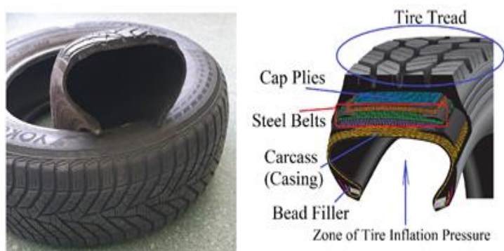
Fig. 1. Composite pneumatic tire construction (based on [6]).
