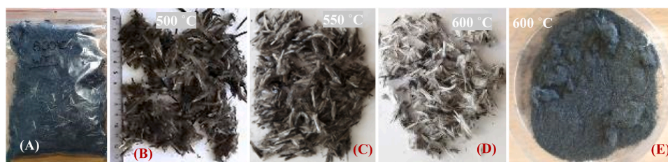
Fig. 5. A) solid residual product, B-D) images of the liberated fibres from solid residual product at 500, 550, and 600°C, respectively and E) char fraction at 600°C.
