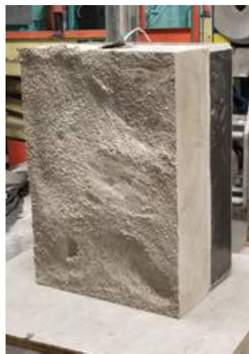
Fig. 2: Sample removed from Wood forms. Note the metal casting that makes up the shell of the panel.
