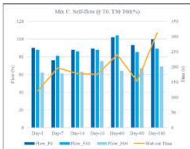
Fig. 6 Impact of ageing on wet-out and flow in Mix-C
