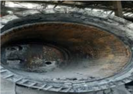
Fig. 7: Ladle condition during dismantling
