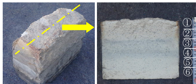
Fig. 4: Appearance and cross section of the developed magnesiaspinal brick used for one year at L/D of 5.8 in a precalciner kiln.
