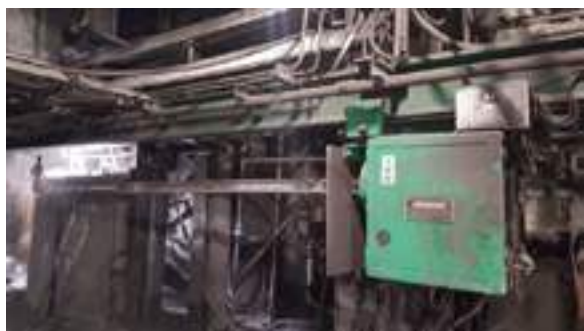
Fig. 1 Stationary ladle gunning installation
