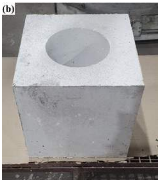
Figure 4: Well block casted from NCC-P mass (a), NCC-P well block after demolding (b)
