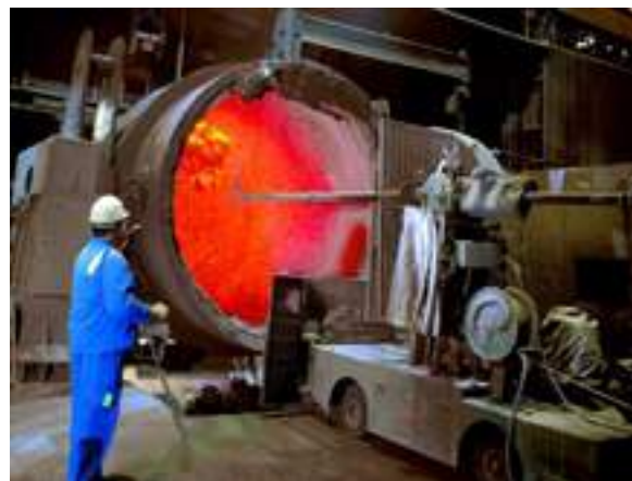
Fig. 2 Mobile lance trolley for ladle gunning
