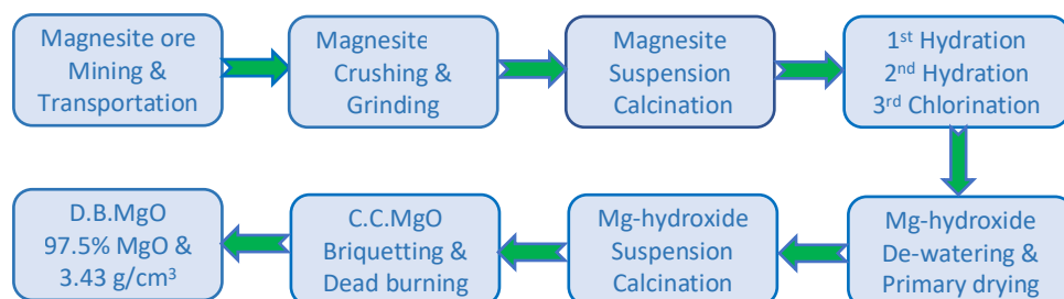
Fig. 1: Flow chart of magnesia purification and densification
