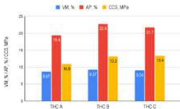
Fig 7 Apparent Porosity (AP), Volatile Matter (VM) and 1300 °C / 3 hrs Cured Cold Crushing Strength (CCS)
