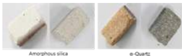
Fig.8 Specimen before and after hydrogen heat treatment
