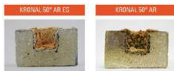
Fig. 8: Alkali resistance of high alumina-SiC bricks with and without application of the ES concept
