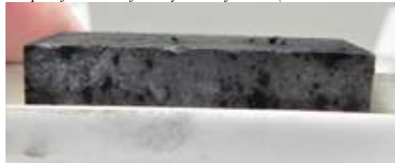
Sample of micropore carbon brick after test (95% CO and 5% H 2 )
