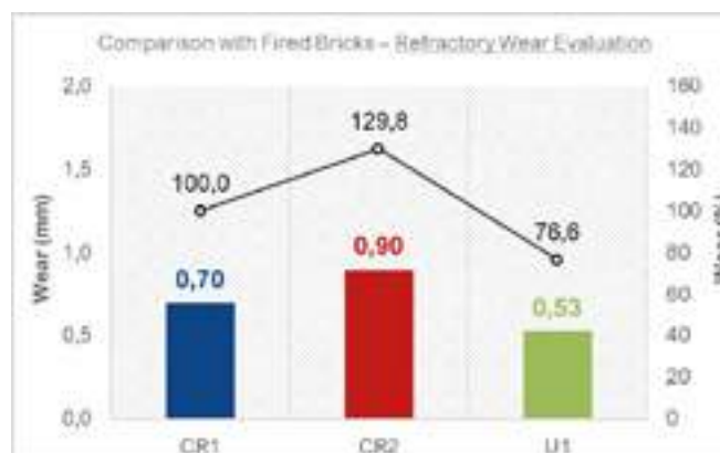
Fig. 3: Absolute and relative wear values after a CaO/Al 2 O 3 rich slag (C2) corrosion test in rotary kiln
