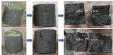
Fig. 4: Status of HTF and LTF brick samples after TSR test.
