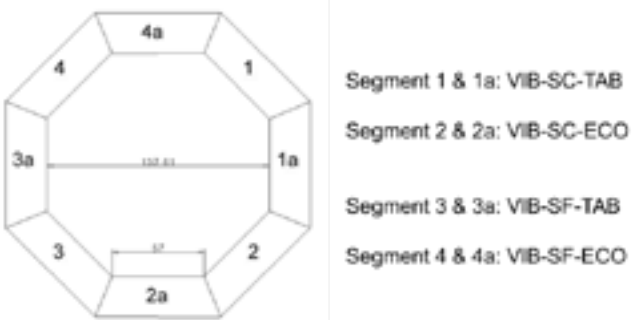
Fig. 9: Schematic drawing of segmentation for the induction furnace corrosion test.
