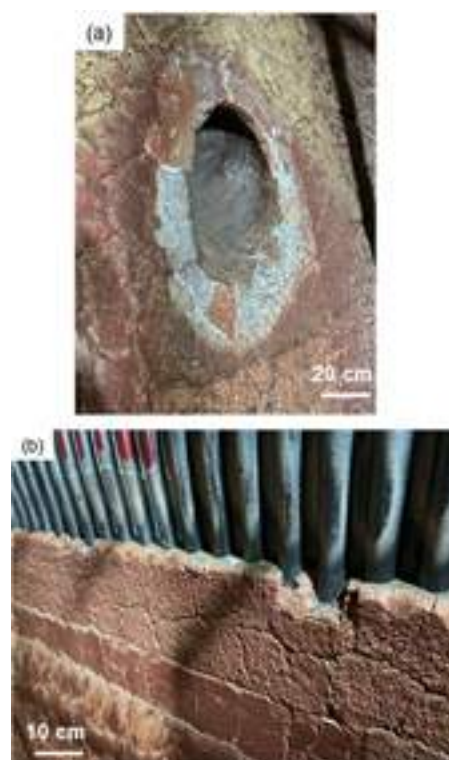
Fig. 2: Erosion wear in (a) the lower and (b) the upper furnace areas.
