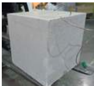
Fig. 4: A 300mm cube with embedded thermocouple in the centre of the specimens to monitor the temperature during the heat-up process.
