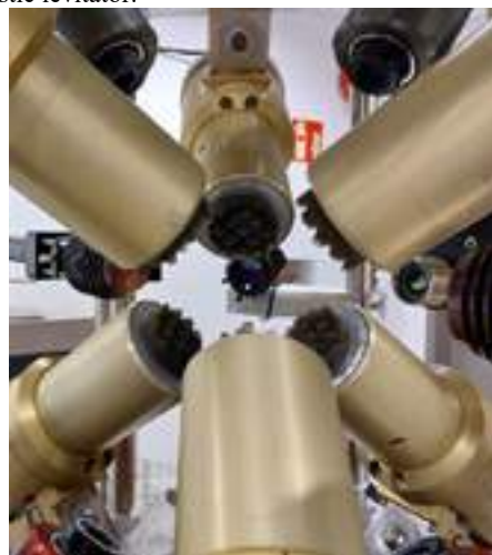
Fig. 1: Aero-acoustic Levitator in operation. An inserted sample is levitating in front of the pyrometer. The golden tubes are ultrasonic transducers.
