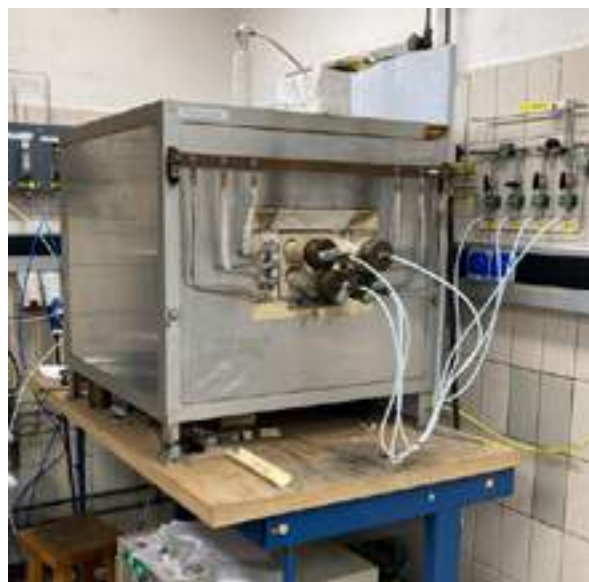
Fig. 3: horizontal tube furnace with gas mixing facilities
