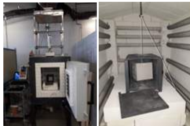
Fig. 3: macro thermogravimetric equipment and sample mounting.
