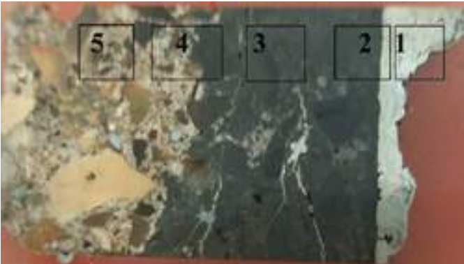
Fig. 2. Photograph showing different regions analysed in the SAMPLE A. 1 – metal area, 2 – metal area/corroded area
