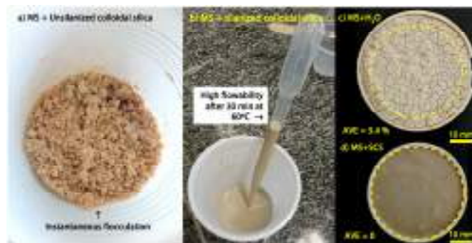
Fig. 1: As-produced aqueous suspensions of MgO sinter with a) unsilanized colloidal silica or b) silanized colloidal silica; samples for AVE measurements (3 days, 60°C, [1]): MgO mixed with c) plain water (MS+ \text{H}_2\text{O} ) or d) silanized colloidal silica (MS+SCS).
