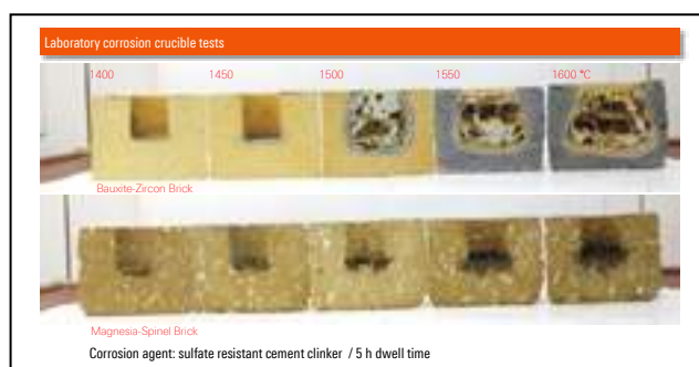
Fig. 1: Cut face sides of crucibles made from aluminosilicate (top) and basic bricks (bottom) after corrosion tests with sulfate resistant cement clinker as corrosive agent.
