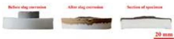
Fig. 7: Corroded CMA cylinder specimen
