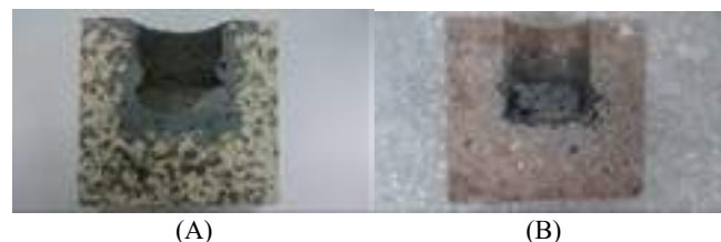
Fig. 1: Comparison of slag erosion by crucible method (A) original high alumina recipe and (B) olivine based recipe B.
