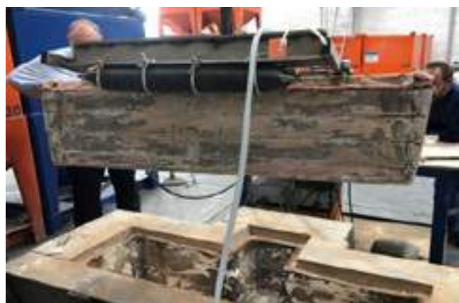
Fig. 5: Baked dry mix in lap test with eMould
