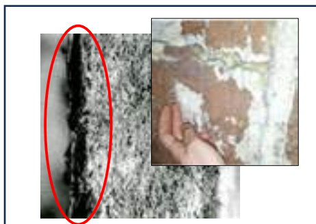
Fig.11. Alteration of ceramic fibres by sulphuric acid after 3 months
