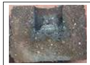
Fig. 10: Mg-Cr (20 % Cr_2O_3 ), slag is completely infiltrated
