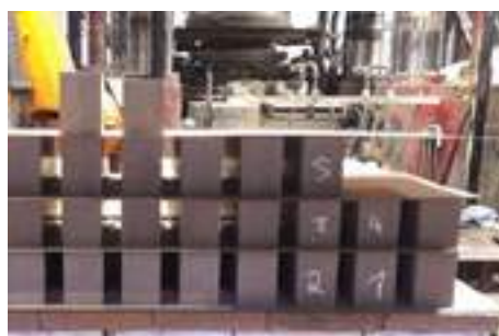
Fig. 5: Pyramid-like setting pattern to prevent bricks from falling and blockage of tunnel kiln. Reprinted from [5] with permission.
