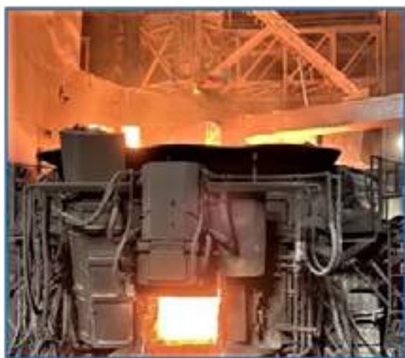
Fig. 3 MINSCAN™ Gunning Head in operation
