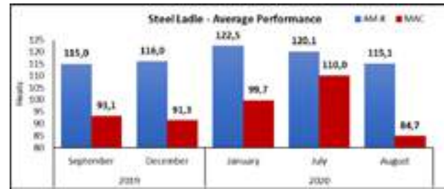
Fig. 2. Average performance comparison between MAC and AM-K lining with the zero carbon technology concept.
