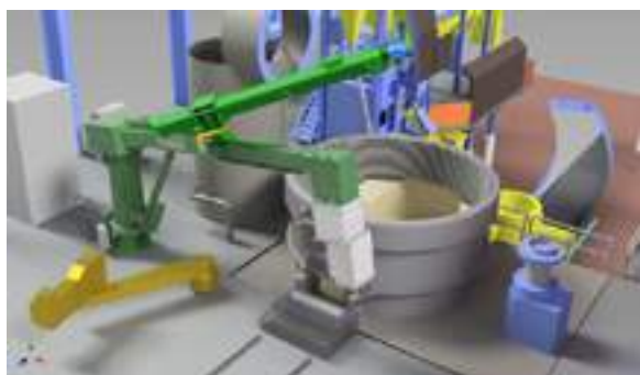
Fig. 8 a, b Gunning robot with laser scanner arm in parking, resp. scanning mode
