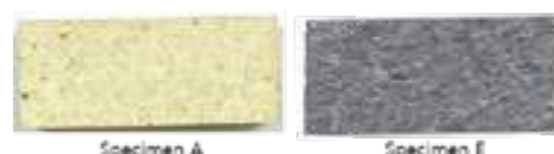
Fig. 2: Specimen before and after hydrogen heat treatment
