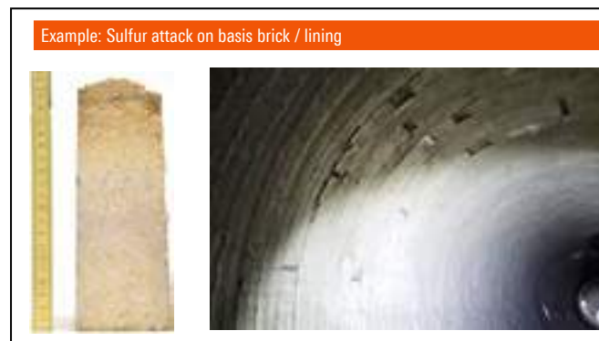
Fig.4: Structural cut face side of a magnesia-spinel brick after use and lining showing signs of sulfur attack.
