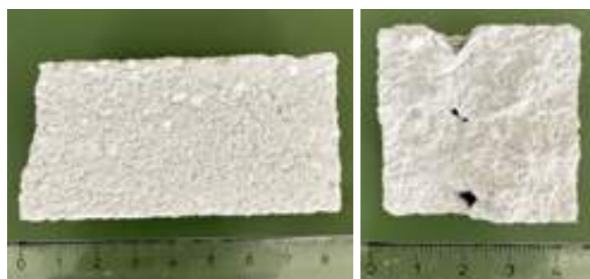
Fig. 6: Cut test piece (180° angle), to show the inner structure of built layer on layer construction in print direction (l.) and fracture surface of cut test piece (180° angle), to show the inner structure of built layer on layer construction (r.).
