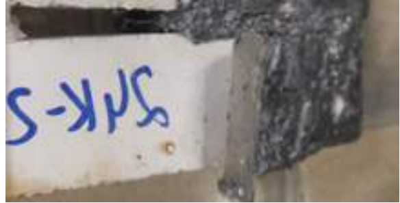
Fig. 1. Macroscopic morphology of castables after corrosion by molten aluminium. SAMPLE A – phosphate bonded bauxite-based castables, SAMPLE B – hydraulically bonded bauxite-based castables, SAMPLE C – hydraulically bonded lightweight refractory aggregates-containing castables.
