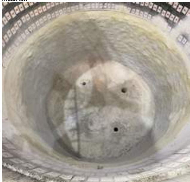
Fig.5: Steel ladle repaired with ShotGun
