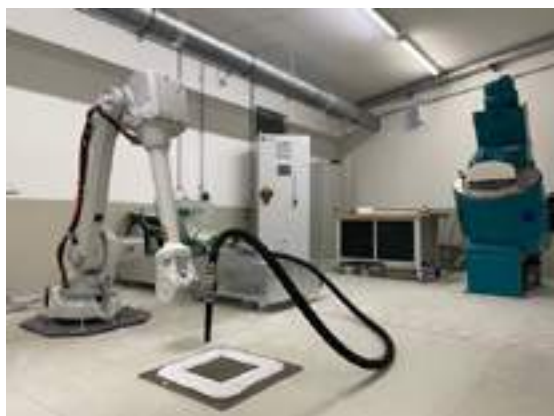
Fig. 1: Process chain of Contour-Crafting (from r. to l.): After homogenization by using an intensive mixer, a concrete pump transports the material to the manipulator to create components weighing up to 400 kg in a three-dimensional space.
