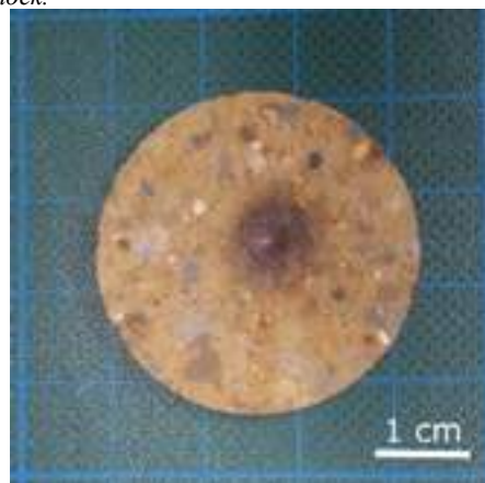
Fig 4: A B80 sample after three rounds of thermal shocks at 1500 °C furnace temperature. At the laser spot, the sample is molten during laser impact and quenched to an amorphous phase after the thermal shock.
