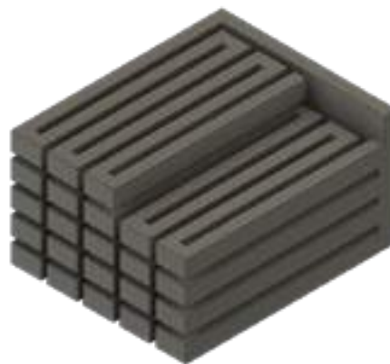
Fig. 2: CAD design of five layers of a cuboid (350 mm x 290 mm). Endless print path without any stoppage of material flow, carried out with a printing path by alignment of the subsequent layers in a 180° angle.
