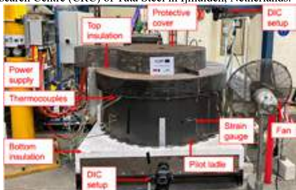
Fig. 3: Experimental setup of the pilot ladle.
