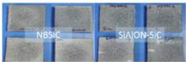
Fig. 6. NBSiC & SiAlON-SiC samples after abrasion test
