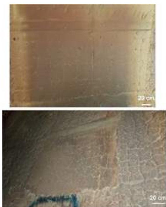
Fig. 9: No relevant wear was identified in the refractory lining (extensive cracks or thickness reduction), after a campaign time of 4 months.
