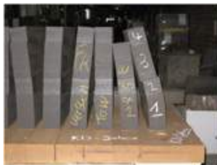
Fig. 4: Severely deformed bricks on kiln car due to high iron levels in raw material. Reprinted from [5] with permission.
