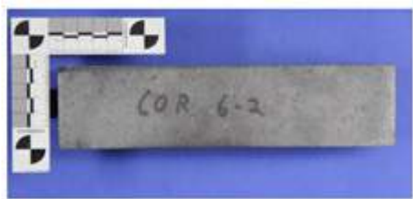
Fig. 4 : NBSiC Unaffected / Class A
