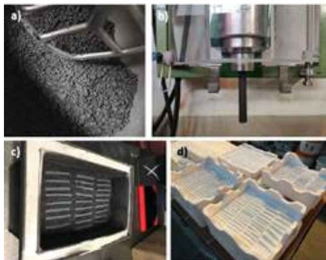
Fig. 1: Sample preparation; a) Extrusion mix in intensive mixer; b) Piston extruder; firing preparation of bar-shaped carbon-bonded samples in pet-coke bed (c) and oxidic samples (d).
