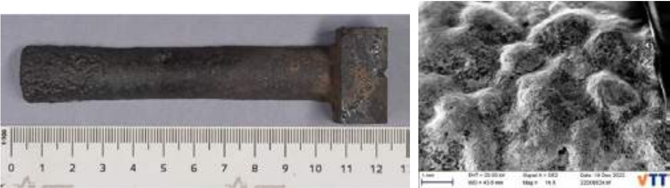
Fig. 3: Refractory finger after testing in slag contact and SEM image of the surface with slag reactions.
