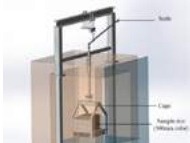
Fig. 3: Schematic drawing of the industrial-scale thermo-balance (Macro-TGA).
