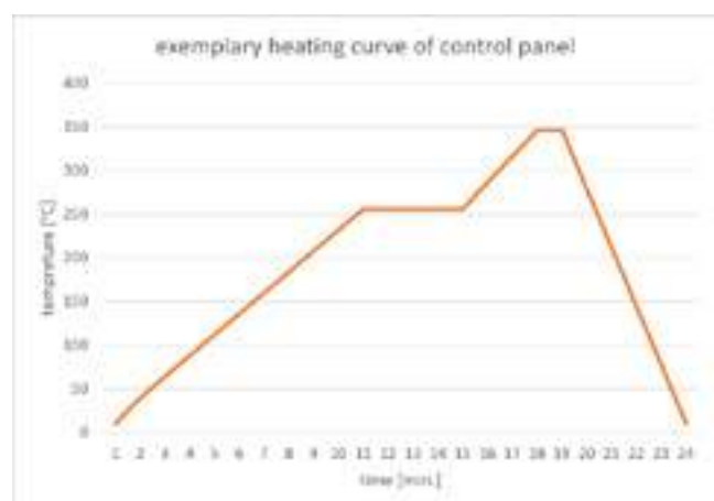
Fig. 3: Heating curve of control panel eMould
