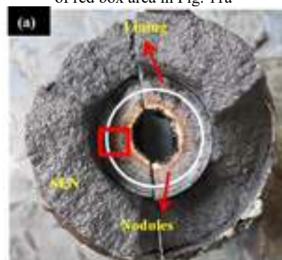
Fig. 6 Fracture morphology of cloggings on \text{Al}_2\text{O}_3\text{-C} specimen when the inner pressure in specimen is 30000 Pa: (a) cross section fracture at the red line mark of specimen; (b,c) enlargement diagram of red box area in Fig. 11a
