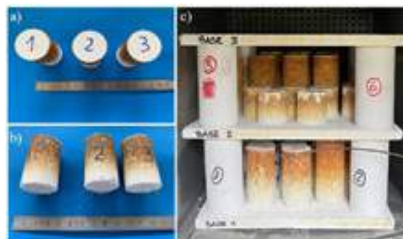
Fig. 1: Photos of pressed refractory samples before the corrosion test. The arrangement of samples inside the furnace is shown in (c).
