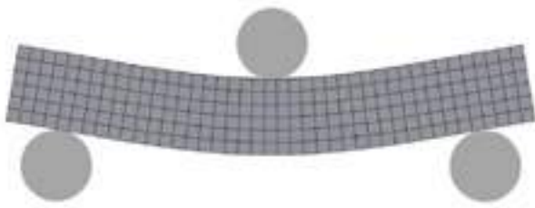
Fig. 5: Illustration of a finite element model of the three-point bending test.
