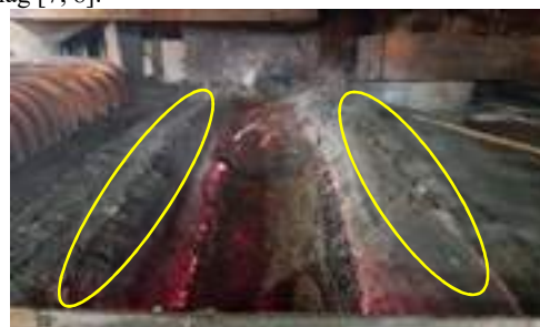
Fig. 1. Slag zone damage during main runner usage
