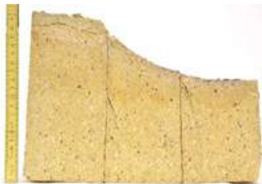
Fig. 1: Thermally eroded alumina lining in the safety zone of a cement clinker rotary kiln. Smoothly and wavy eroded brick surfaces can be observed in the foreground. Transition to the basic lining in outlet direction is marked with a dashed line.
