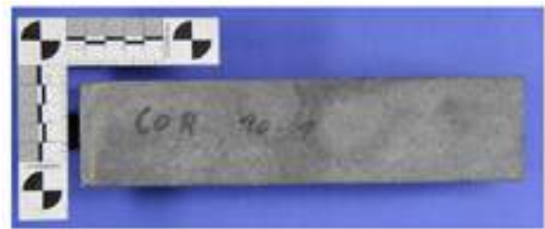
Fig. 5 : SiAlON-SiC Unaffected / Class A
