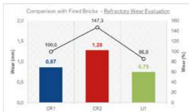
Fig. 2: Absolute and relative wear values after a FeO rich slag (F2) corrosion test in rotary kiln
