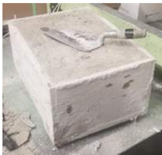
Fig. 1: Gunned sample formed inside shotbox
