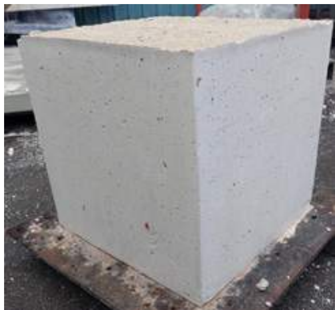
Fig. 7: Element after 16-hour drying time with 0.5 wt-% CAC content.
