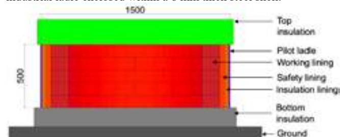
Fig. 1: Graphical illustration of the pilot steel ladle showing pilot ladle, refractory linings, and top and bottom insulation.
