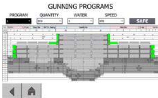
Fig. 5 Zone selection for automatic gunning
