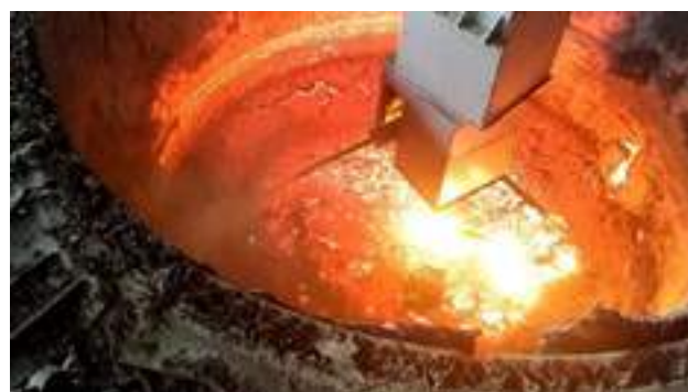
Fig. 7 hot gunning repair with PNEUTOP
