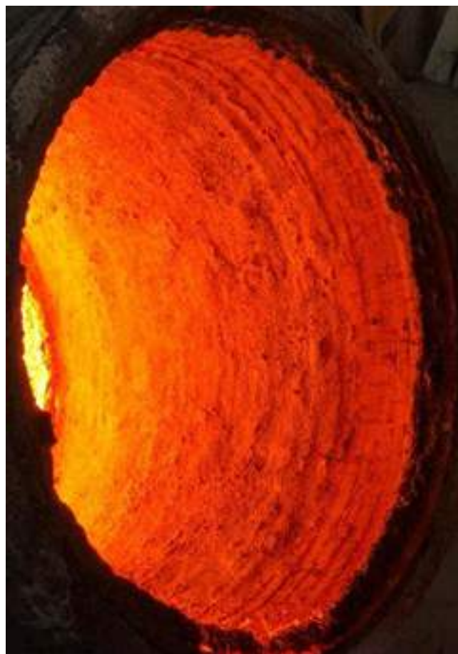
Fig. 6: Steel ladle repaired with ShotGun during operation
