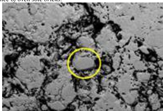
Fig. 10: Special additive grain in KS quality bricks; increases abrasion resistance of oven sole bricks.
