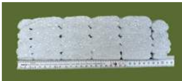
Fig. 5: Cut cuboid, to show the inner structure of built layer on layer construction against print direction.
