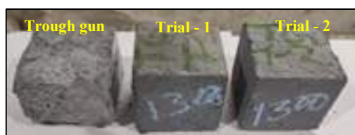
Fig.3: Samples appearance after blasting test at 1300°C
