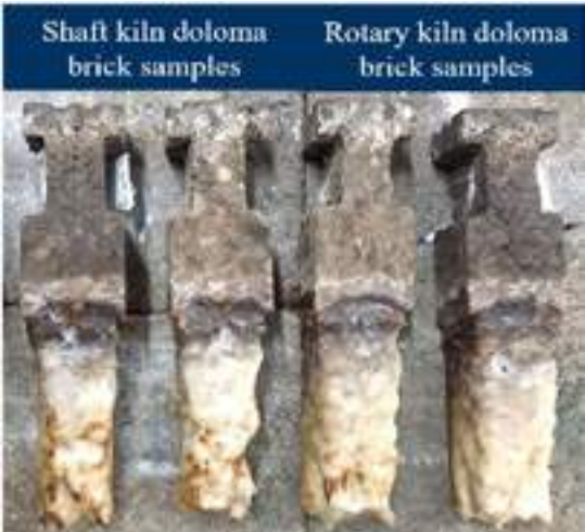
Fig. 7: Finger-shaped slag testing samples after slag corrosion tests. Brick samples prepared with shaft kiln doloma material (left) and rotary kiln doloma having higher bulk density and lower silica levels (right).
