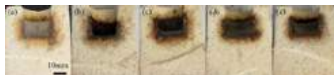
Fig. 7: Images of cross-section of the corroded samples X0 (a), X2 (b), X4 (c), X6 (d) and X8 (e)
