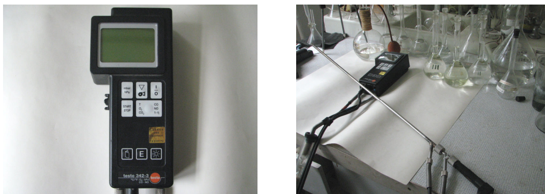
Fig. 2.4 Gas analyser TESTO 342-3 (Germany)
