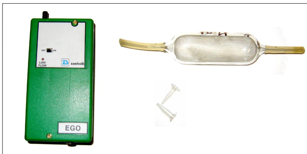
**Figure 2.3.** Sampling equipment: 1 – sampling pump, 2 - gas pipette, 3 – plugs.
