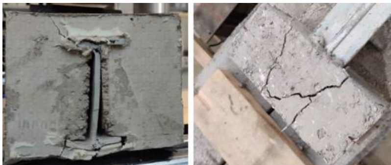
Fig. 3.15. Typical failure of the support block of the first series beam (made by the author)
