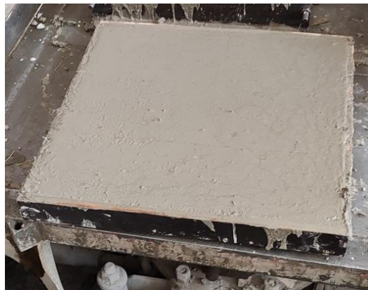
Fig. 3.4. Casted PFRC plate (made by the author)
