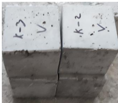
Fig. 3.10. 100 mm cubes cast after every beam series (made by the author)
