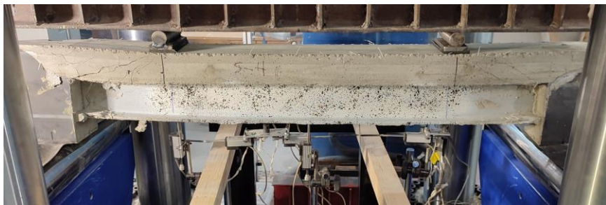
Fig. 3.17. Tested the second series hybrid beam prototype (made by the author)
