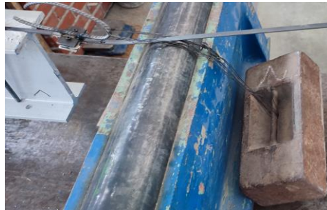
Fig. 3.24. Prestressing mechanism (made by the author)
