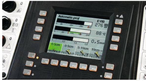
Fig. 18. Roller operator display with Evib, temperature and amplitude parameters
