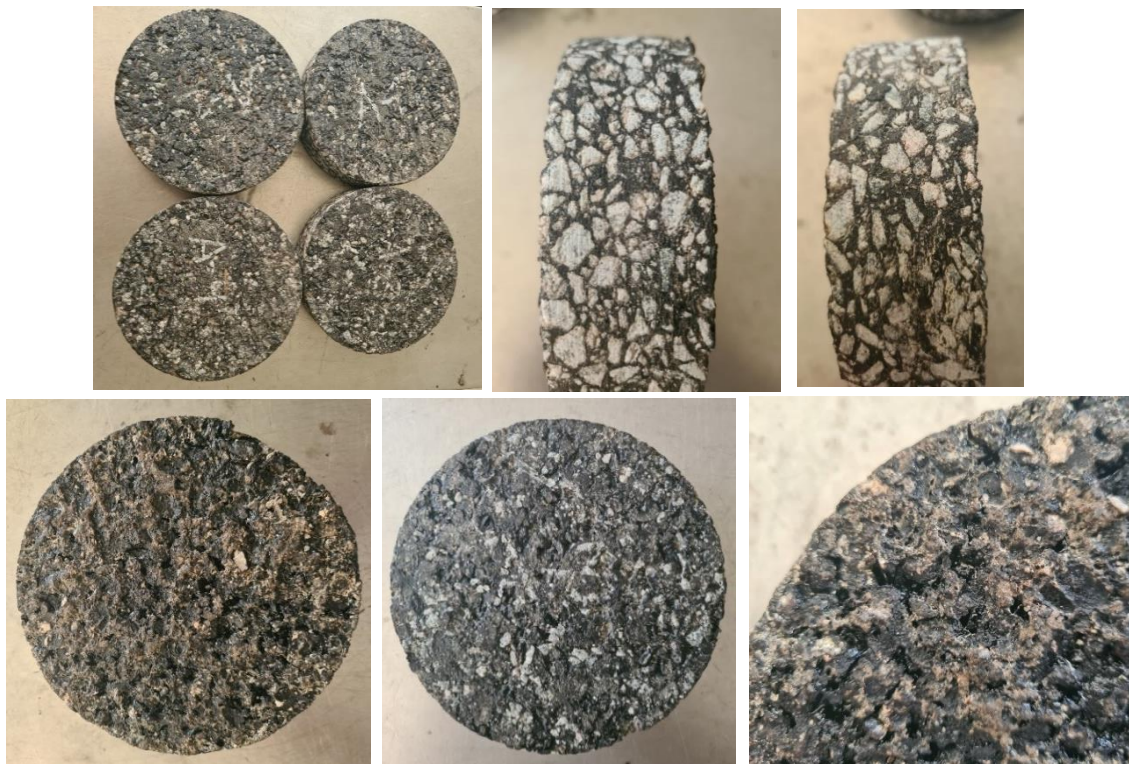
Fig. 35. Extracted cores and their visual density, compaction, and air voids
