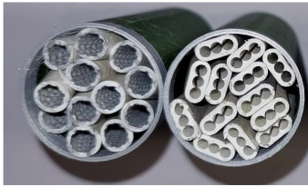
Figure 4. Round structures with cable sheathing filling
