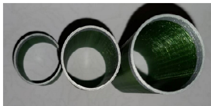
Figure 3. 3D printed tubes in heights of 3 cm, 7 cm, 10 cm
