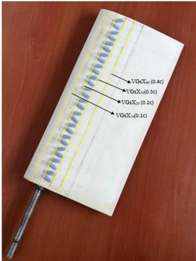
Figure 5: Location of XVGs on NACA 0012 airfoil
