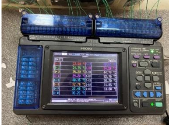
Figure 10. Temperature values read on the display of the data logger
