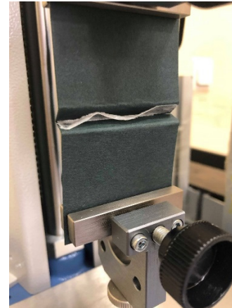
Fig. 4. Test results of samples made from paper “Rives tradition” 170 gsm. a) Unsticking/tearing results at 1 \text{ mm min}^{-1} stretching speed; b) Specimen at the end of the test.
