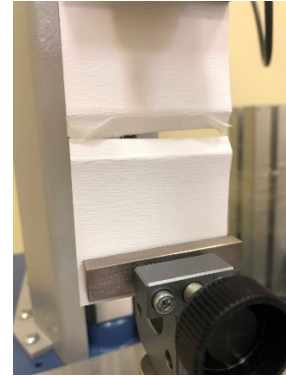
Fig. 4. Test results of samples made from paper “Rives tradition” 170 gsm. a) Unsticking/tearing results at 1 \text{ mm min}^{-1} stretching speed; b) Specimen at the end of the test.
