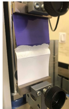
Fig. 6. Test results of samples made from glossy laminate “Deprosa”: a) Unsticking/tearing results at 1 \text{ mm min}^{-1} stretching speed; b) The specimen made from glossy laminate bonded with hot glue, during the test.
