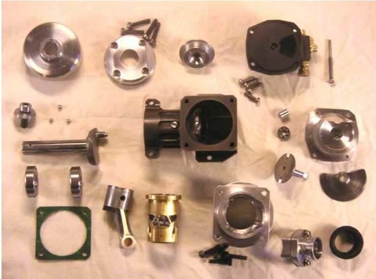
Figure 4.1.3 Disassembled two-stroke engine of tether model car
