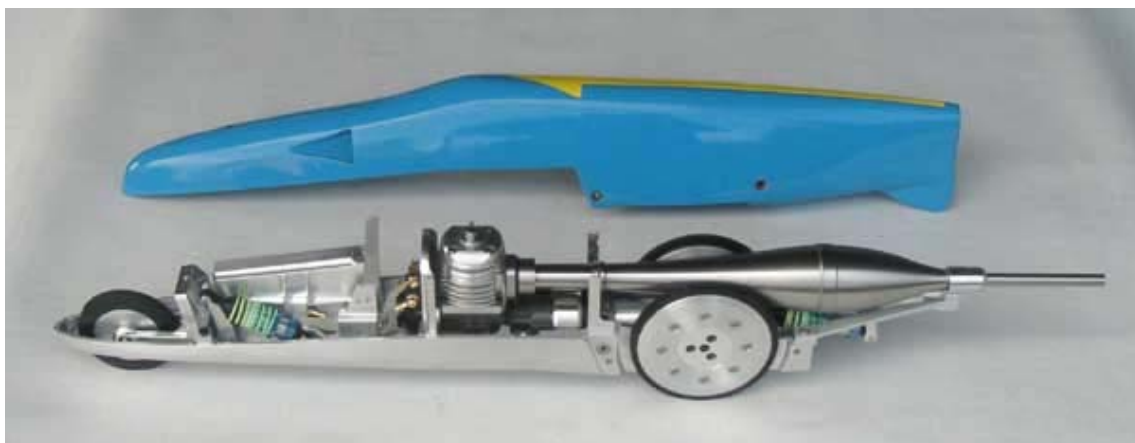
Figure 2.3.2 Tether race car model with removed cover. The engine connected with expansion chamber.
