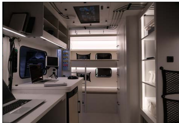
Fig. 5. Overview of the interiors of the rigid trailer unit: meal preparation area with storage on the left, crew quarters in the background and hygiene compartment access door on the right. Rack laboratory and working tables in the front.
