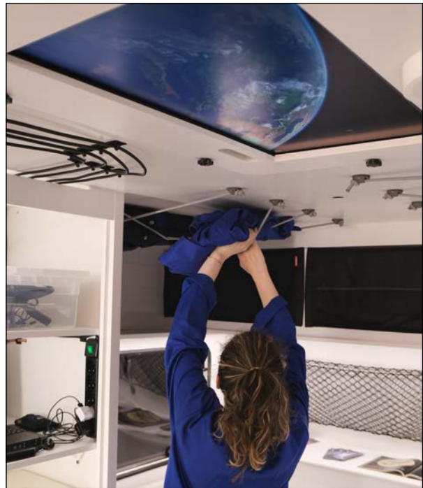
Fig. 7. Ceiling storage solutions and virtual displays both to optimize storage capacity and also to simulate the spatial perception experienced in the ISS.
