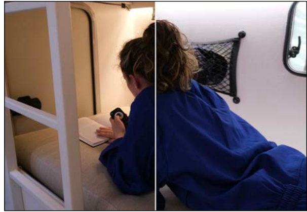
Fig. 12. Smart Lighting System in Solar Light Mode with Warm or Cool Light Spectrum to replicate daylight conditions at different times of the day and positively reinforce circadian rhythms. Remotely controllable from the Mission Control.
