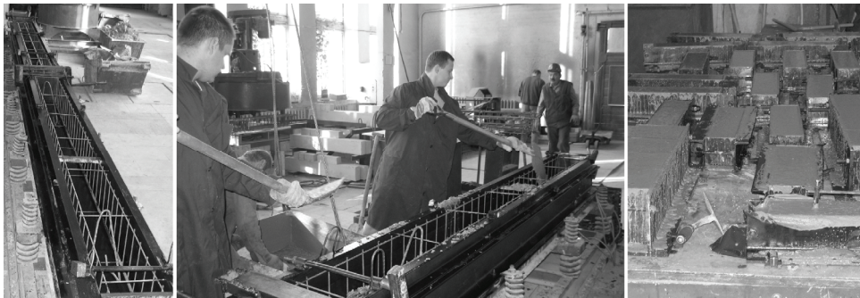
Fig. 3.3. Casting the beams and test specimens
