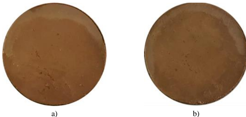
Fig. 3.16. The surface of the clay composite after the water erosion test: a) RSH-2.5(3) composite; b) RSH-2.5(5) composite
