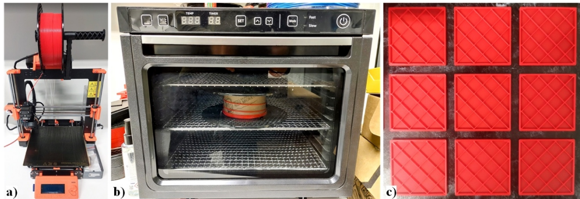
Fig. 1. Additive production: a) 3D printer, b) filament dryer, c) cross-section of the specimens.
