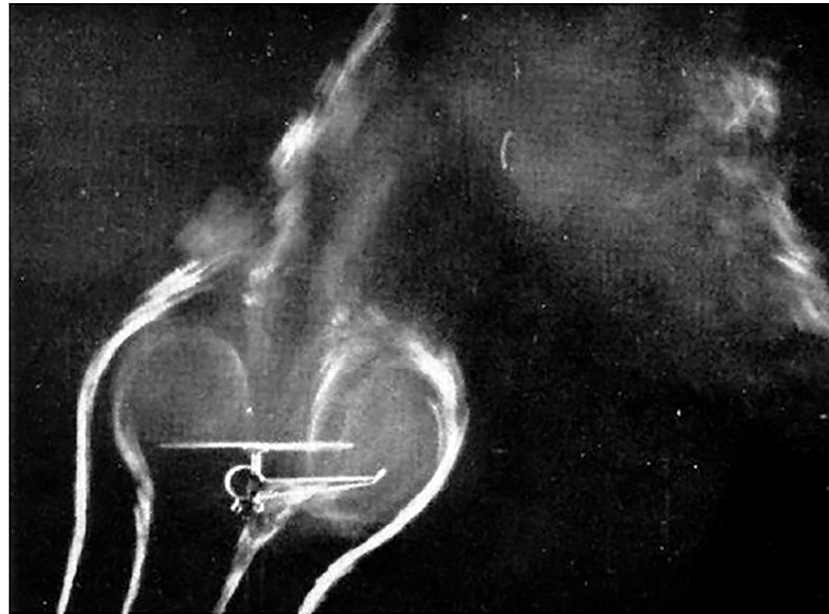
Figure 1. Visualization of the Vortex Ring State (VRS) [8].
