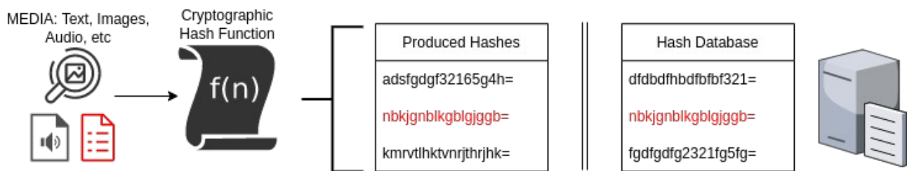
Figure 1: Process of media being hashed and compared against a hash database
