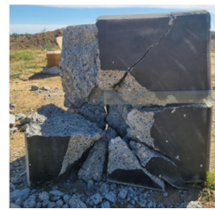
Fig. 4 Concrete block after impact
