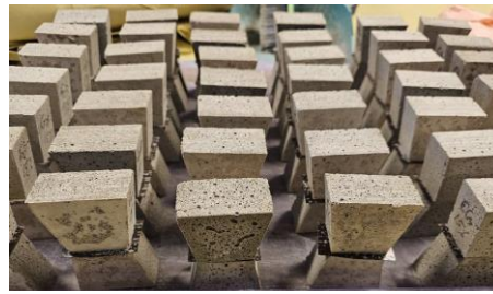
Fig. 2. Concrete specimens ready to be tested
