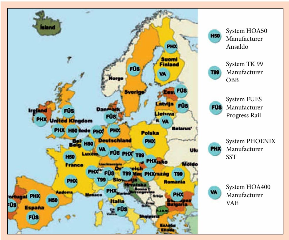
Figure 10. Hot axle-box detection systems in Europe Railways (Eisenbrand 2011)
