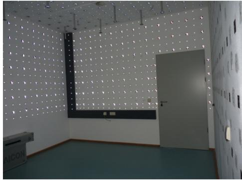
**Fig. 6.1.**Test-field for the camera calibration
