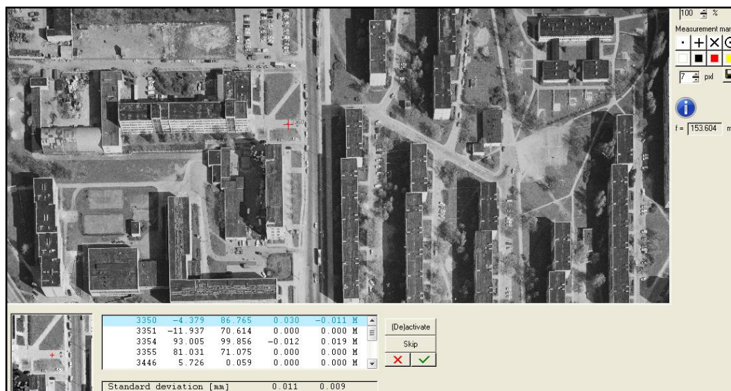
Figure 3. Processing of aerial photography using digital photogrammetric system ( LISA )
