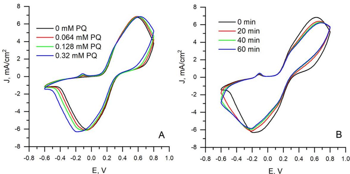
**Figure 4.** (A) Cyclic voltammograms at different concentrations of PQ. (B) Cyclic voltammograms at different time intervals with 0.32 mM PQ. The working solution was 19.23 mM potassium ferricyanide in PBS. The scan rate of  $0.1 \text{ V s}^{-1}$  and potential step of  $0.01 \text{ V}$  was applied.
