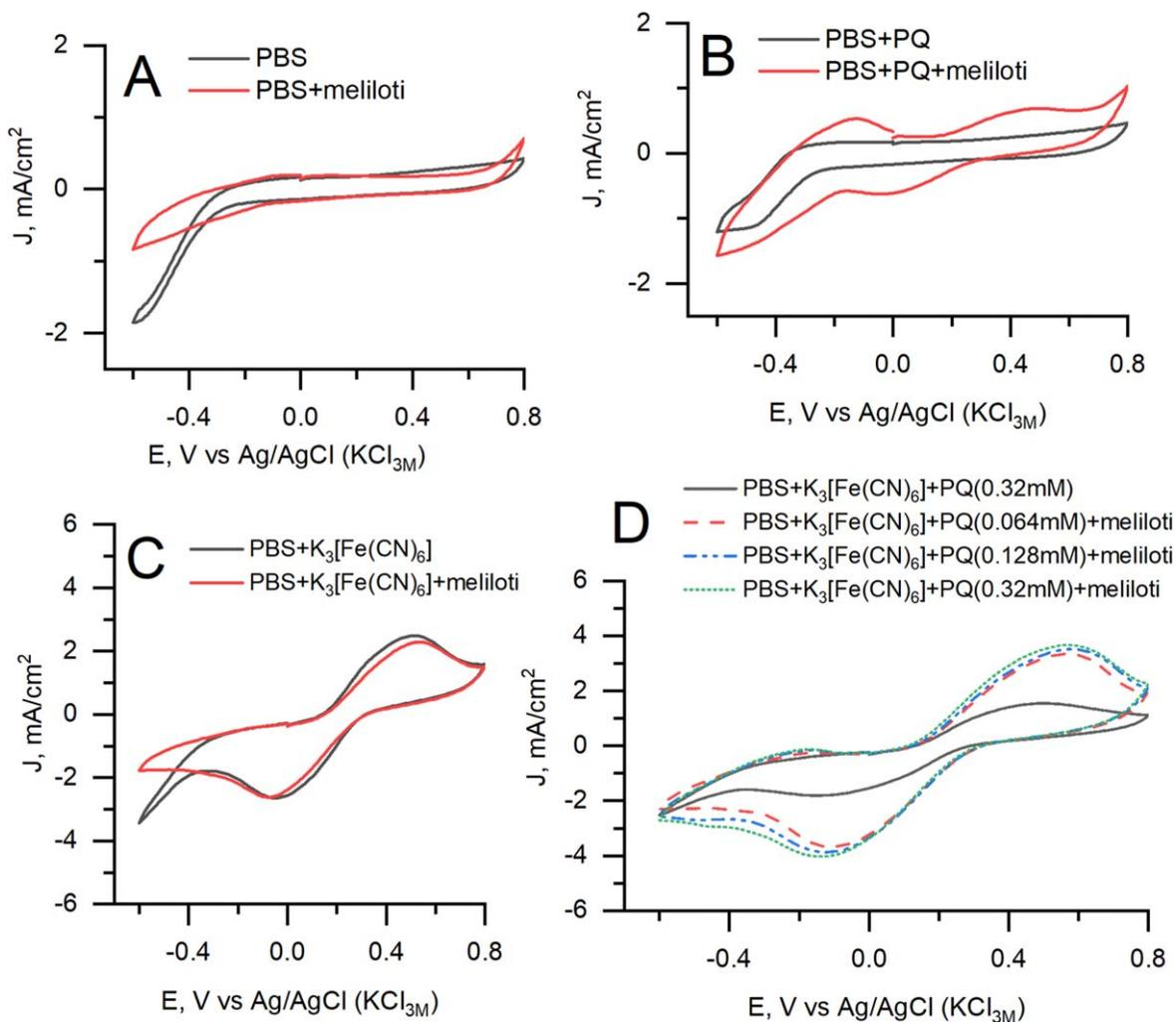
**Figure 3.** Cyclic voltammograms with and without *E. meliloti*. (A) in PBS. (B) in PBS with 0.32 mM PQ. (C) in PBS with K<sub>3</sub>[Fe(CN)<sub>6</sub>]. (D) in PBS, 19.23 mM K<sub>3</sub>[Fe(CN)<sub>6</sub>], and different PQ concentrations. The scan rate of 0.1 V s<sup>-1</sup> and potential step of 0.01 V was applied.
