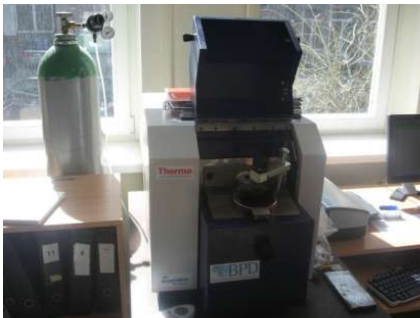
18 pav. Thermo Scientific ARL QuantoDesk spektrometras
