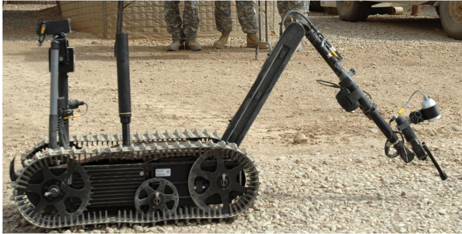
1.7 pav. „Talon“ 2 DOF” manipulatorius (Talon – Qinetiq... 2012)
