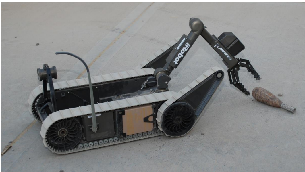
1.5 pav. iRobot “PackBot” mobilusis robotas (The U.S.... 2009)
