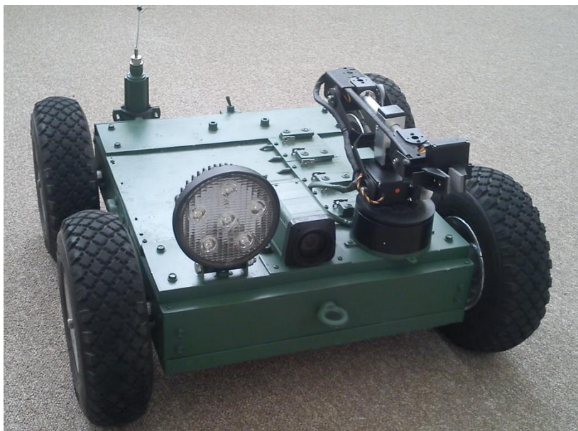
1.10 pav. Tiriamasis manipuliatorius ant mobiliojo roboto
