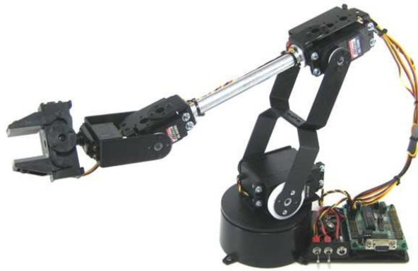
2.2 pav. Tiriamasis elektromechaninis manipulatorius (AL5D Robotic... 2014)
