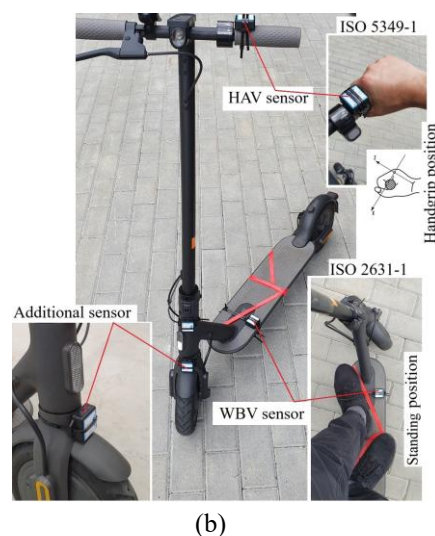
Fig. 6. Main experiment of the research: (a) Instruction of ride; (b) E-scooter equipped for measuring.
