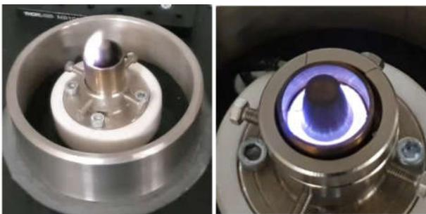
Figure 2. Plasma stabilisation with permanent magnets
