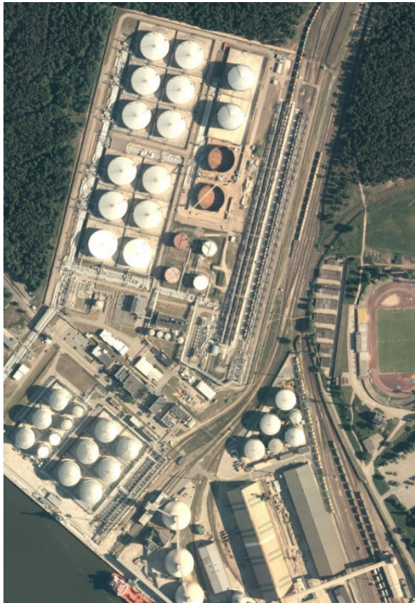
Fig. 2.3. An example of exposure of an industrial facility to the hazard of a railway tanker BLEVE: railway tracks coming along tank farms in the port of Klaipėda (obtained with maps.lt software)
