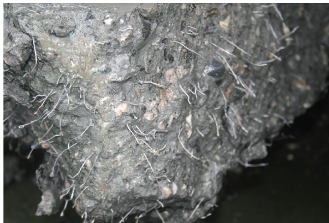
Figure 5: Fracture surface of steel fibre-reinforced concrete (Bischo., 2007)
