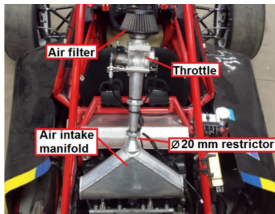
Fig. 2. Formula Student engine air intake manifold with Ø20 mm air restrictor.
