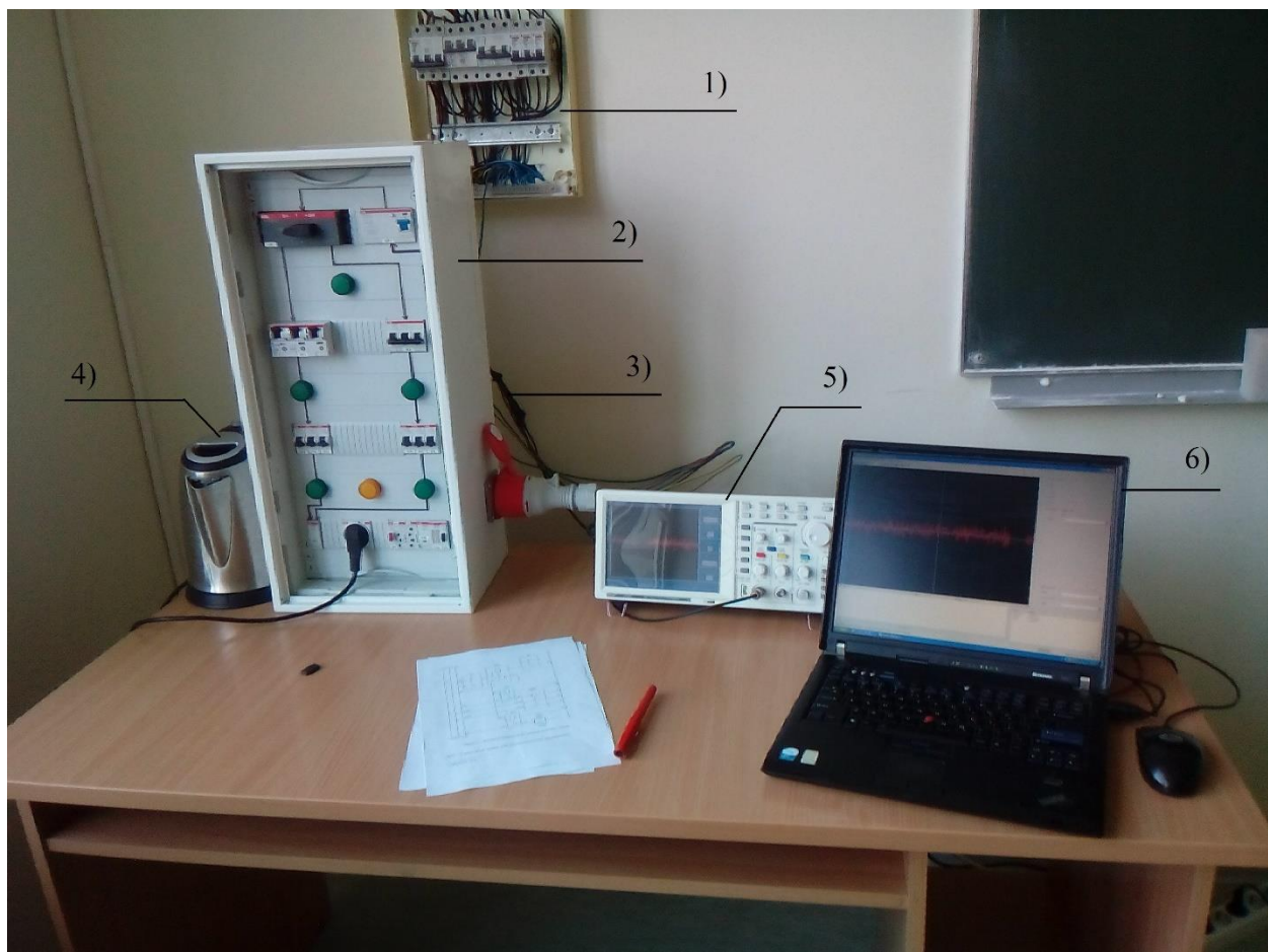
Figure 3.1 – Equipment for conducting the experiment, where 1) – connection point to the power grid of the building; 2) – short circuit stand; 3) – Hall effect sensor; 4) – 2kW electric load (electric kettle); 5) – digital storage oscilloscope; 6) – laptop for data analysis.
