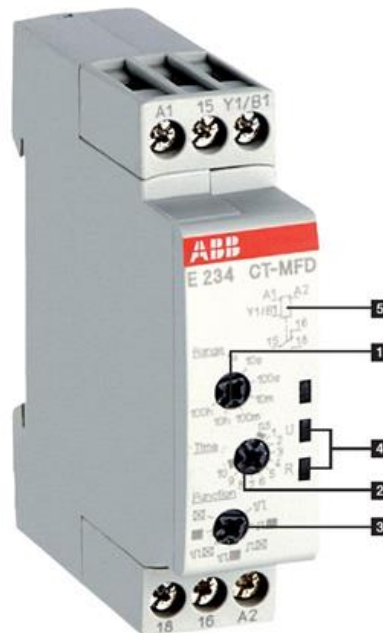
Figure 3.5 – LR1 time relay view with control panel settings explanations, where 1) – rotary switch for the preselection of the time range; 2) – potentiometer with direct reading scale for the fine adjustment of the time delay; 3) – rotary switch for the selection of the timing function; 4) – indication of operational states; 5) – circuit diagram. (ABB STOTZ-KONTAKT GmbH 2007a).
