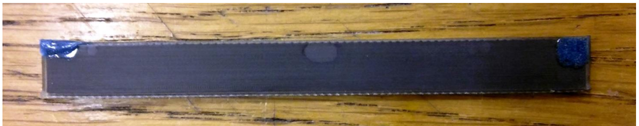
Fig.41 #5 specimen. Complete and sealed with acetone.
