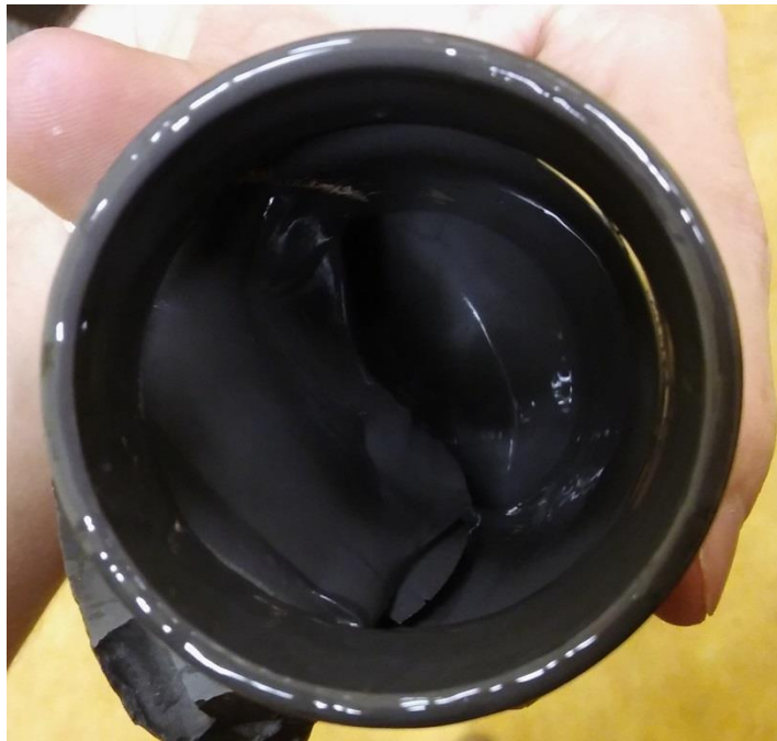
Fig.23 MR fluid inside a container with applied external magnetic field.
