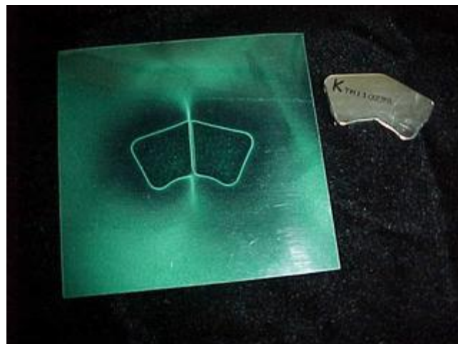
Fig.18 Magnetic field of HDD actuator magnet [25].
