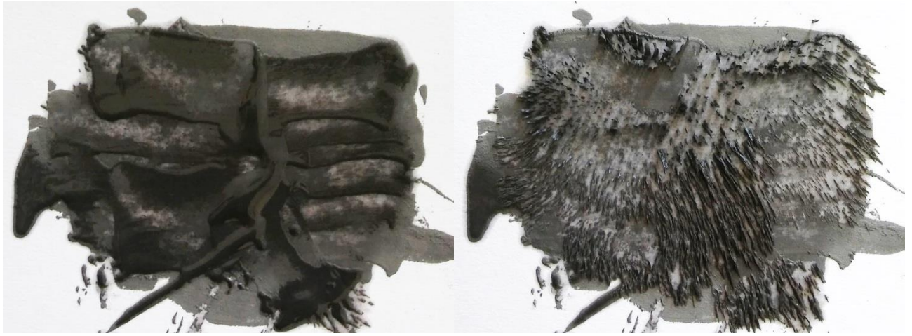
Fig.9 Magnetorheological fluid: without external magnetic field – (left), with external magnetic field – (right).
