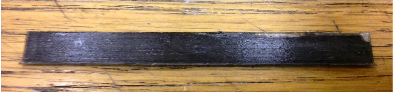
Fig.40 #4 specimen. Successful with insignificant faults. Side view.
