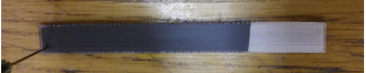
Fig.43 MR fluid being manually injected into specimen.
