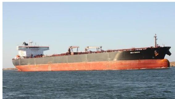
Fig. 1 POST PANAMAX tanker “SEAMAGIC”: L = 250 m, B = 44 m, T = 14,5 m, DWT = 115000 t
