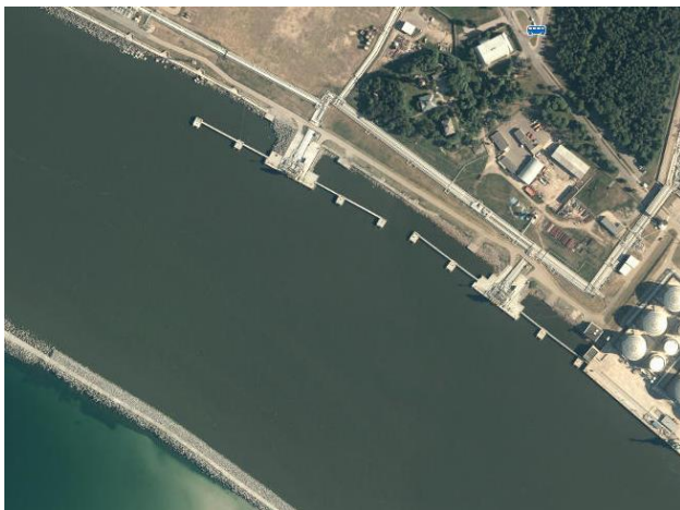
Fig. 4 Klaipeda port oil terminal and its jetties which has length 268 m each, depths near jetties up to 15,5 m
