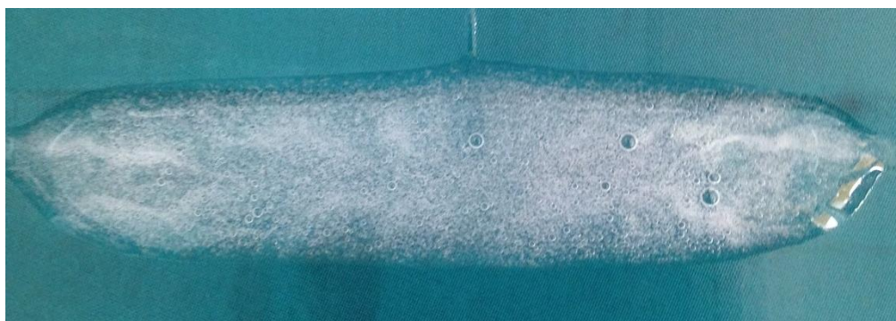
Figure 19 Electrolyte mixture after printing with screen printing (using screen mesh)
