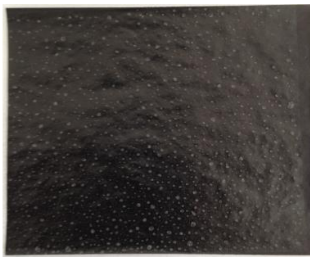
Figure 18 Electrolyte (1:1) printed with screen printing method on G2 with carbon ink layer
