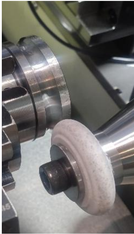
Fig. 5. Sanding the inner part of the bearing
