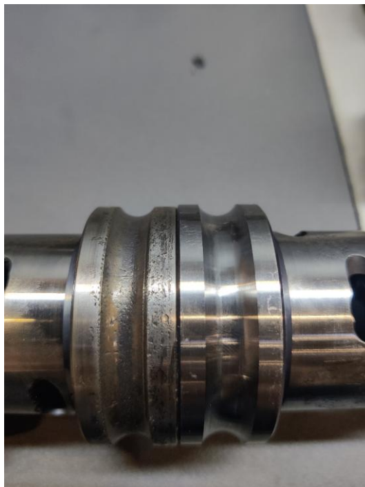
Fig. 4. Under the left rusty inner part of the bearing. Under the right-repaired inner part of the bearing.
