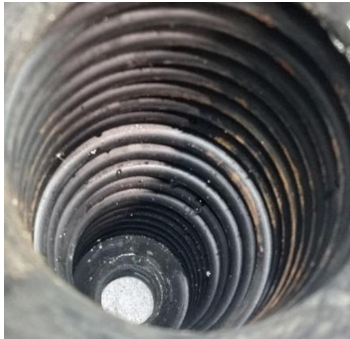
Fig. 2. Protective rubber with moisture entering.
