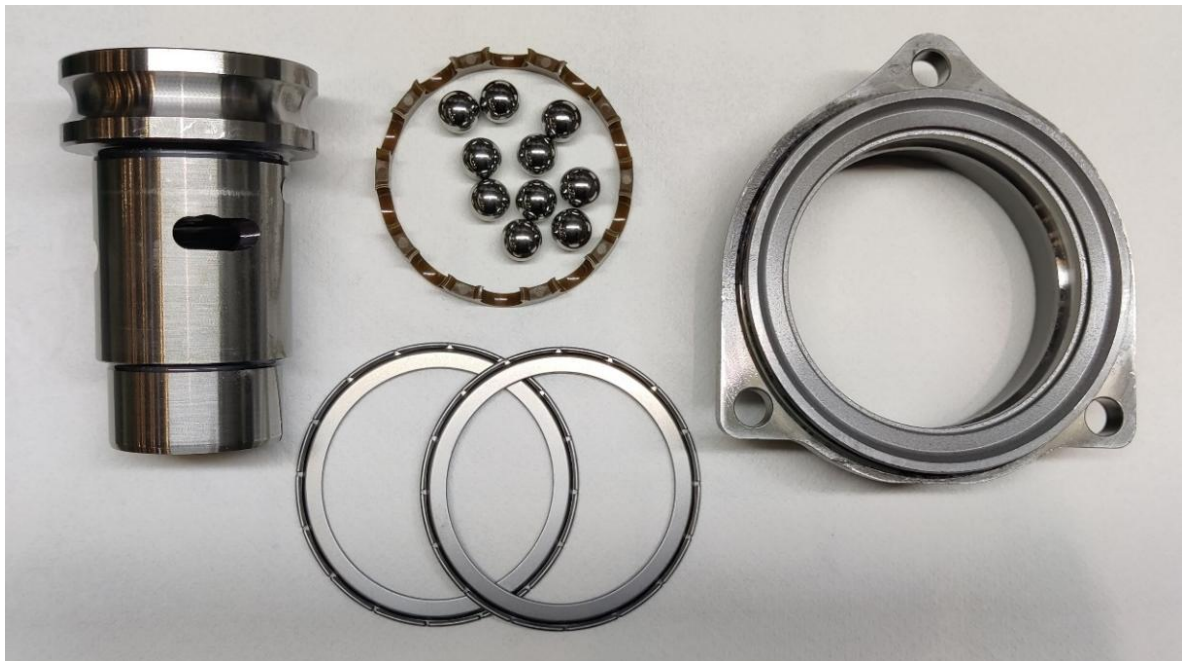
Fig. 6. Prefabricated bearing with new details
