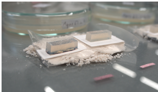
Figure 1. Preliminary tests of an agar gel poultice with calcium phytate on sample paper over a mineral clay substructure.
