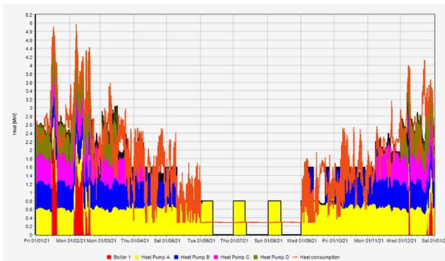
Figure 26. Stage-1 Heat Production
