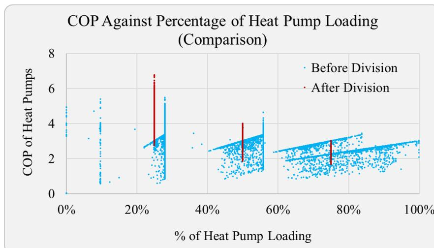
Figure 43. Comparison of COP on HP Loading (Before Vs After Network Division)
