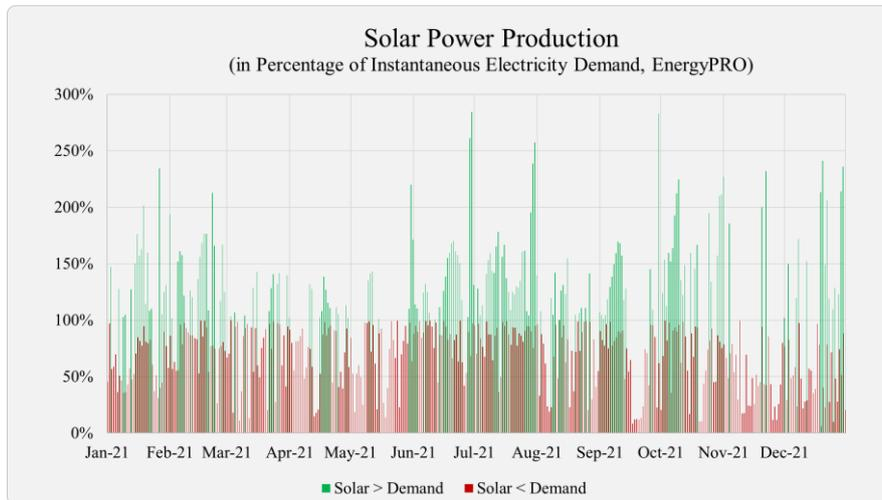
*Figure 40. Stage-2 Hourly PV Solar Power Production for 2021 (Compared with Electricity Demand)*
