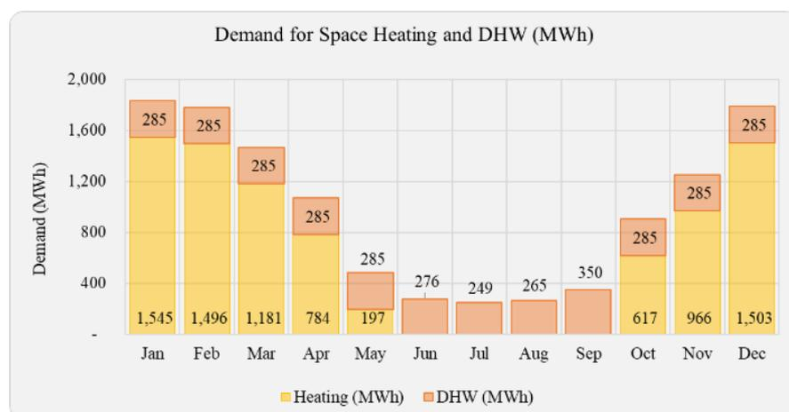
Figure 5. Segregation of Demand - Space Heating and DHW (2021)
