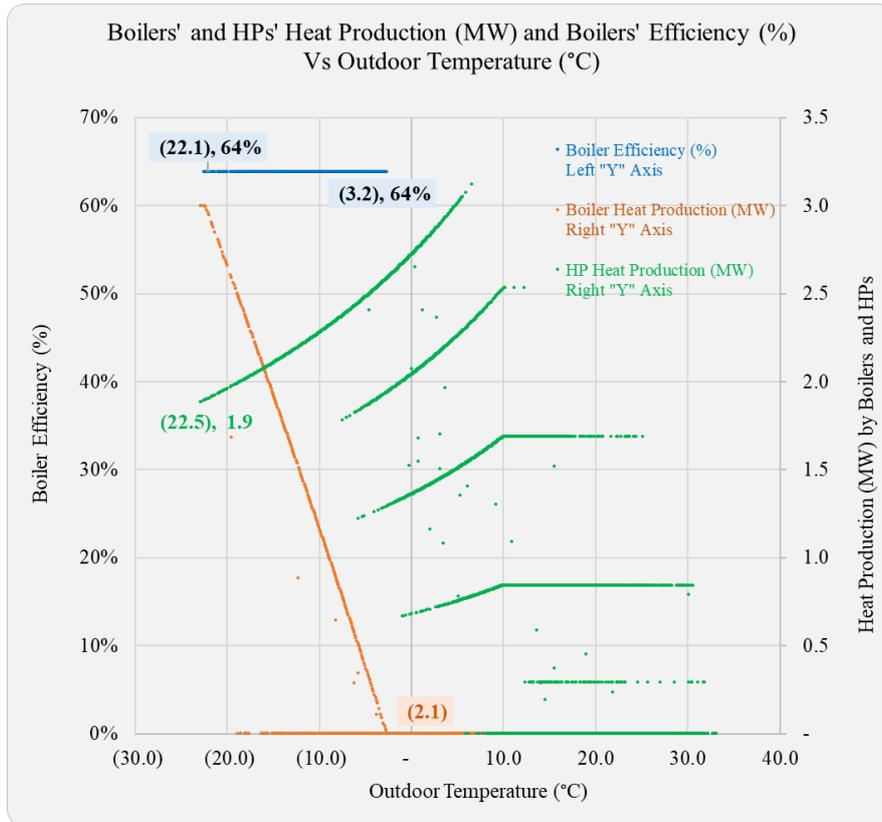
Figure 39. Stage-1 Heat Production (MW) by Boilers & HPs, and Boiler Efficiency Vs Outdoor Temperature
