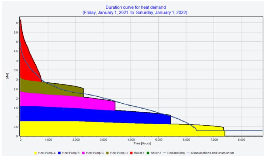
Figure 28. Stage-1 Duration Curve
