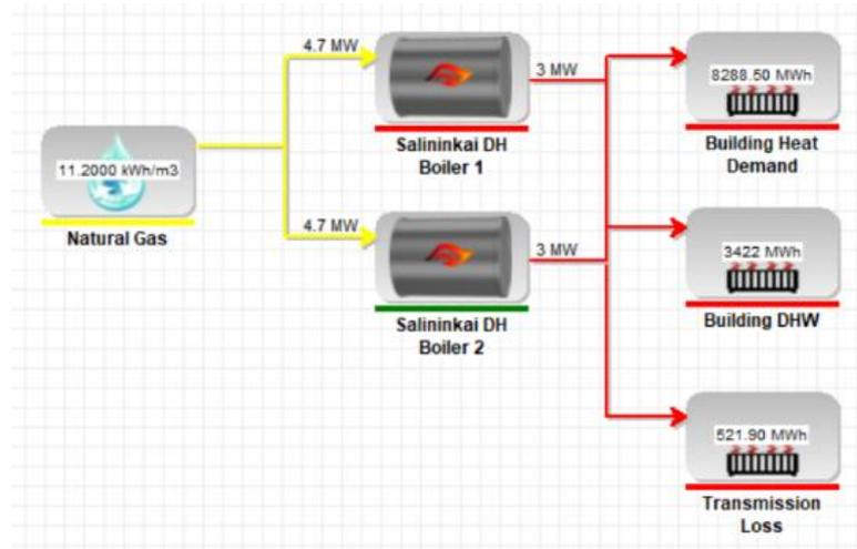
Figure 8. Baseline System (Existing Setup)
