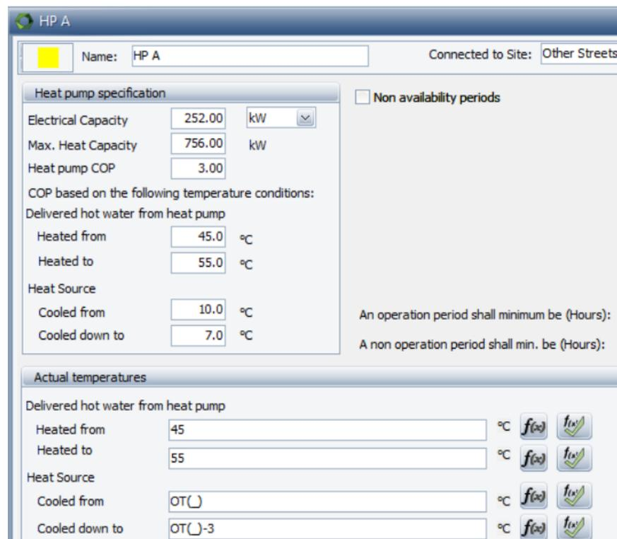
Figure 10. EnergyPRO Input Parameters for Heat Pumps
