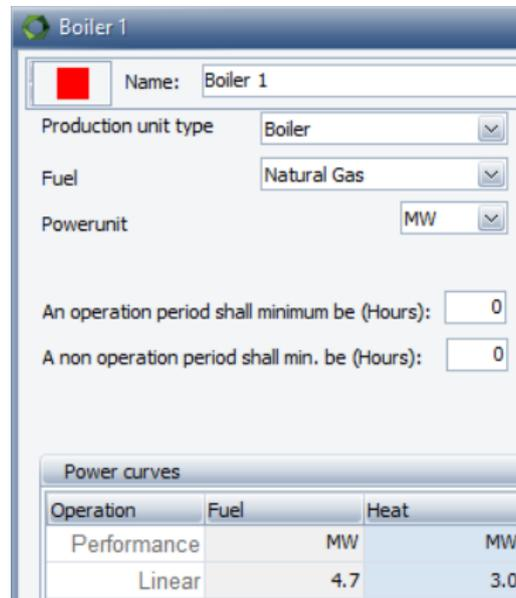
Figure 9. EnergyPRO Simulation Input Window of Boiler-1
