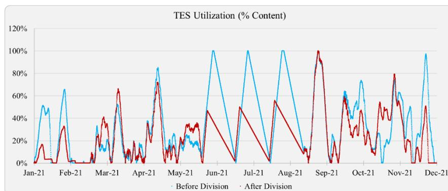
Figure 45. TES Utilization (Before and After Network Division)
