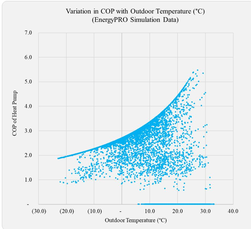
Figure 38. Stage-1 Variation of Heat Pumps' COP
