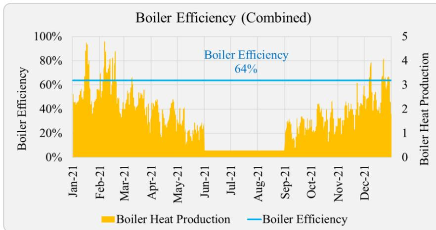
Figure 25. Baseline - Boiler (Combined) Heat Production and Efficiency
