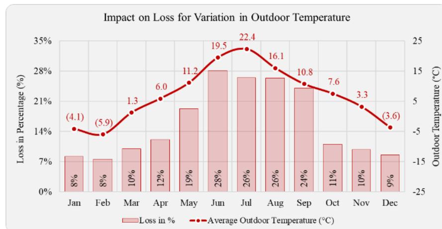
Figure 3. Monthly Loss (2021) Variation with Outdoor Temperature
