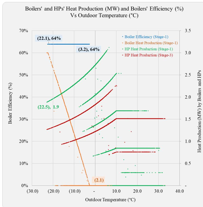
Figure 44. Comparison of Heat Production (Stage-1 Vs Stage-3)
