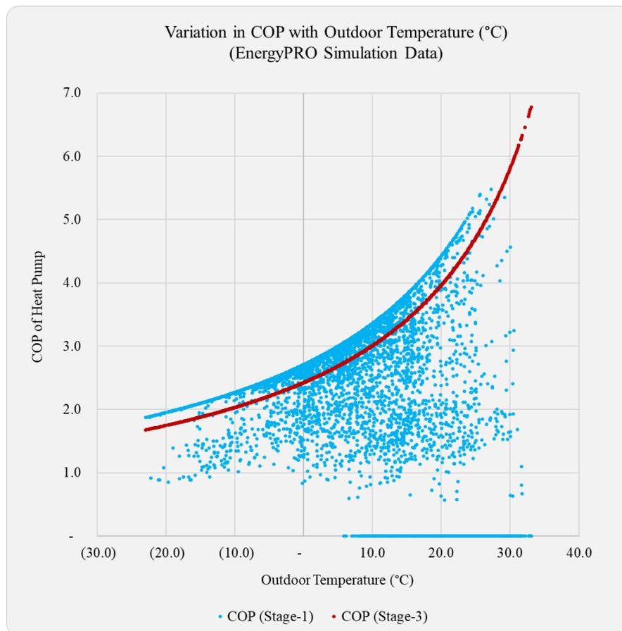
Figure 42. Comparison of HPs' COP (Before Vs After Network Division)
