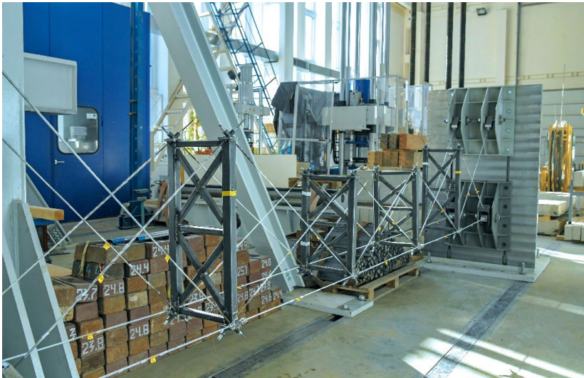
Fig. 3.1. Model of cable-stayed string bridge
