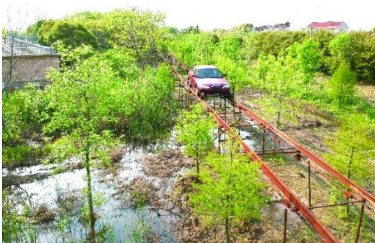
1.7 pav. Bandomasis AERORail modelis (Li et al., 2023) Fig 1.7. Test of AERORail model (Li et al., 2023)
