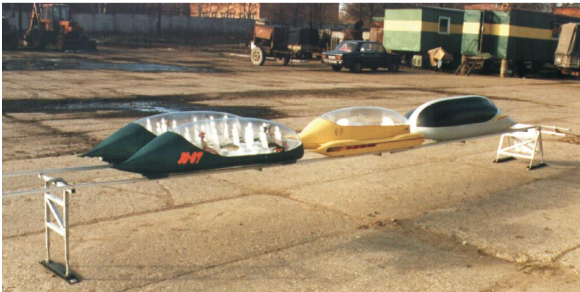
1.5 pav. Styginio transporto bandomieji modeliai (Unitsky, 2008) Fig. 1.5. String transport test models (Unitsky, 2008)
